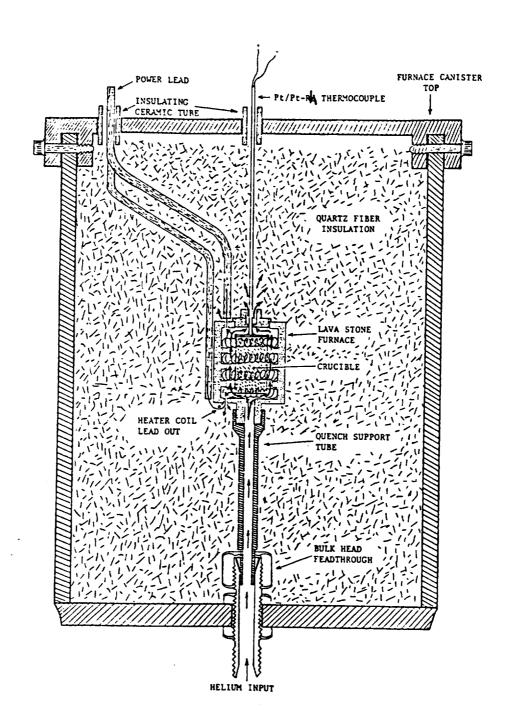
Figure 2. Details of the of the crucible and sample geometry
