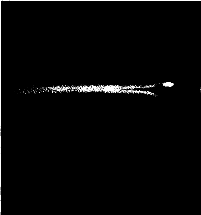
Figure 10. Seven frames from the start of pyrolysis, the plume looks fully developed and laminar. This image is 233 msec from the pyrolysis start, and 733 msec from the start of the current in the wire.
