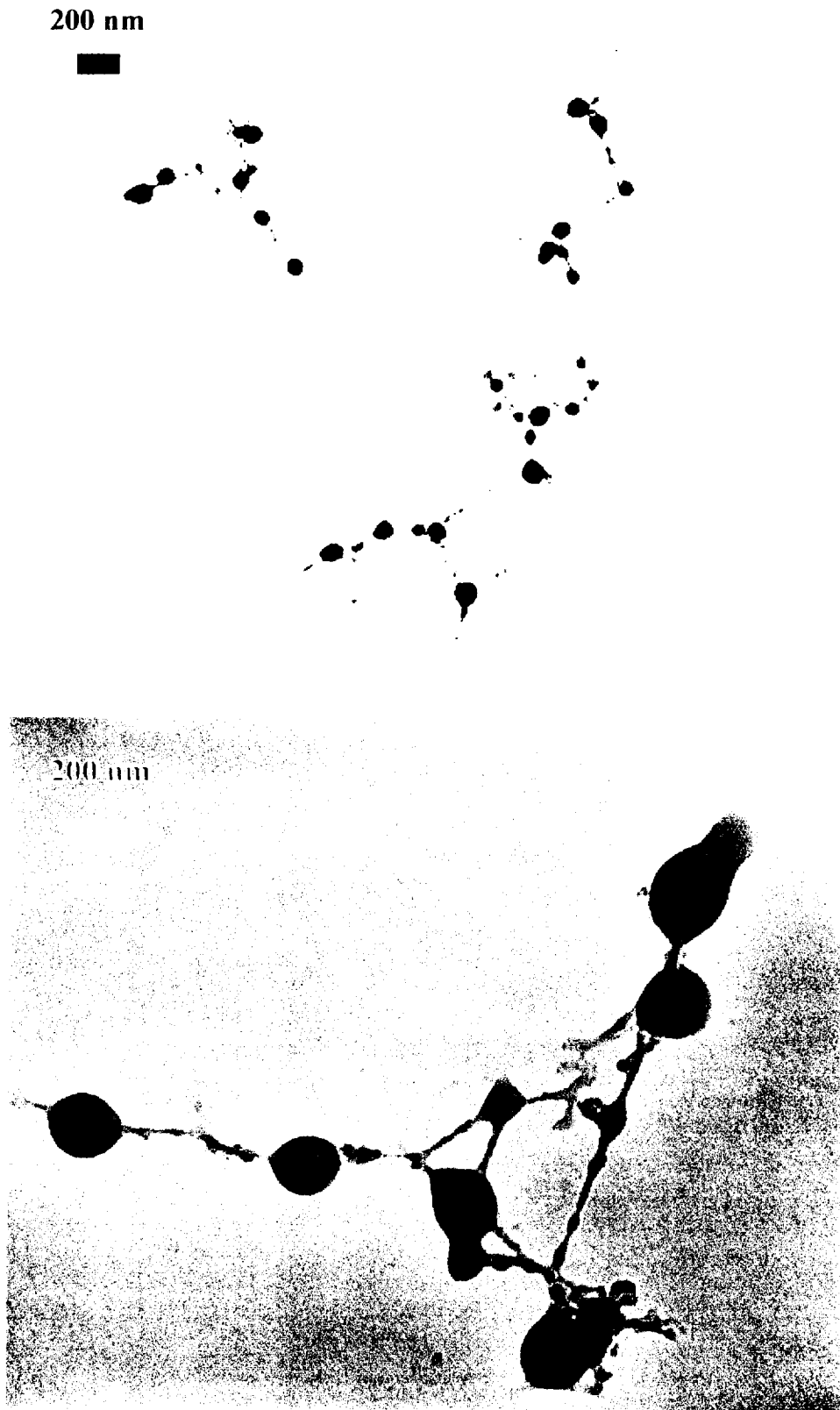
Figure 26. TEM micrographs of particles from red Teflon wire under microgravity.
