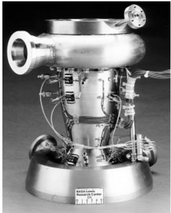
High-aspect-ratio cooling channel combustion chamber.
