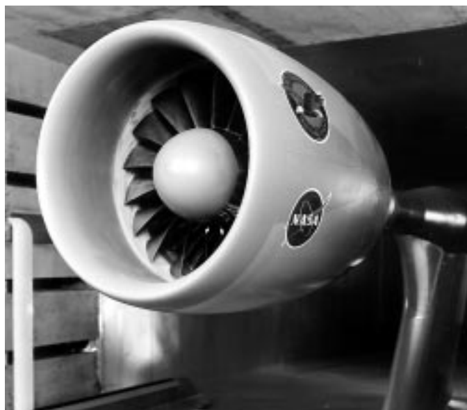
Low-tip-speed fan installed in wind tunnel.
