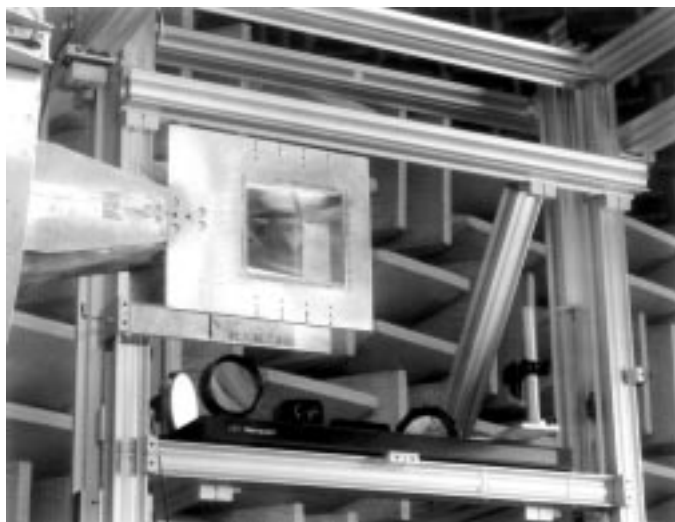
Ejector nozzle being used to study mixing processes for noise reduction.
