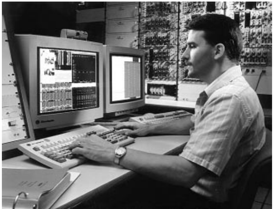
Remote Access Control Room being used in a recent test at the Abe Silverstein 10- by 10-Foot Supersonic Wind Tunnel.
