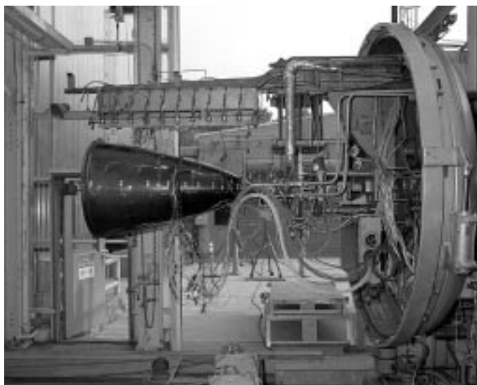
High-area-ratio nozzle on test stand.
