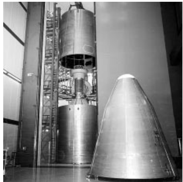
Assembly of the payload fairing in the acoustic chamber, with spacecraft simulator and acoustic blankets for Phase Two testing.
