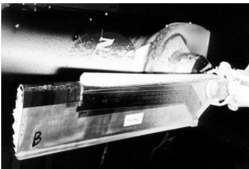
SMA-based deicer mounted on powered rotating rig in Lewis' Icing Research Tunnel.
