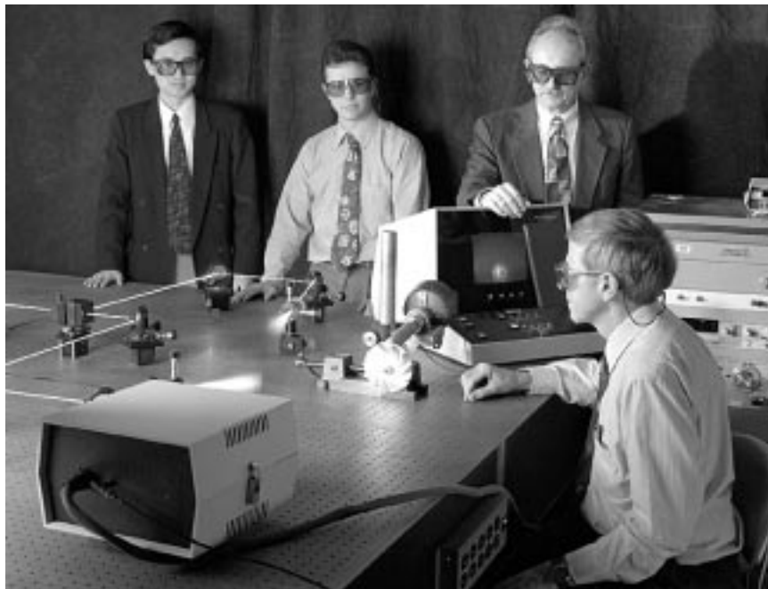
A laser beam is used to study the Kirby G-4 fan in the Lewis Holography Test Lab. From left to right are Kirby engineer Dennis Du, consultant Greg Stewart, and Kirby Senior Vice-President of Research and Development John Lackner. Seated is the Chief of Lewis' Propulsion Systems Branch, Edward Hronek.
