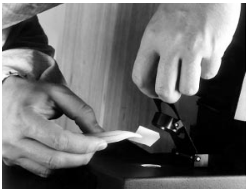
Aperture shield sample being installed in a UV-VIS-NIR (ultraviolet-visible-near infrared) spectrophotometer for optical properties evaluation.
