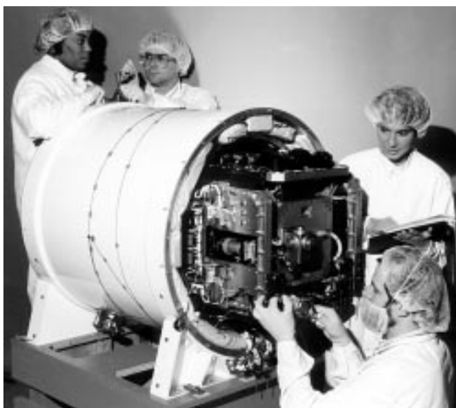
Members of the Lewis-based IDGE team assemble the flight unit. One of the IDGE 35-mm cameras and the Space Acceleration Measurement System (SAMS) sensor head are visible. IDGE is fully operable by remote control from Earth—this feature contributed to its remarkable success on STS-62.
