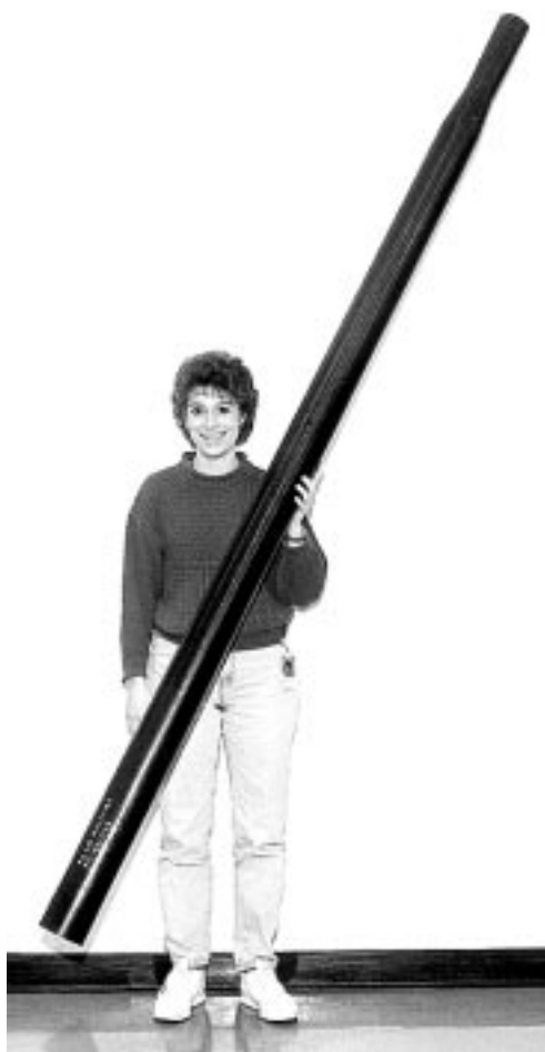
Resin transfer molded AMB-21 Center Vent Tube for the GE-90 engine.
