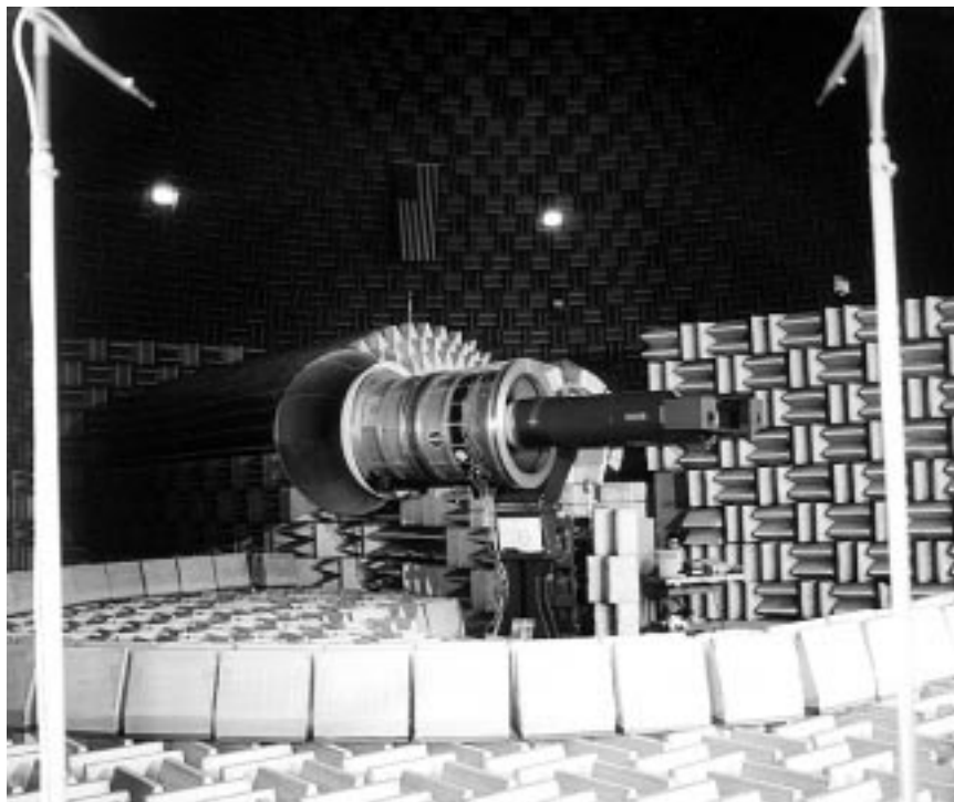
General Electric Company's active noise control system installed on the 4-ft low-speed fan in Lewis' Aero-Acoustic Propulsion Laboratory.
