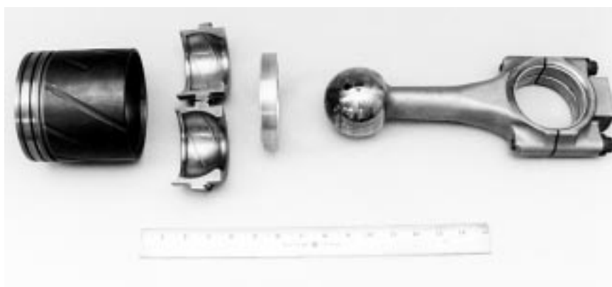
Spherical joint piston and connecting rod—exploded assembly.
