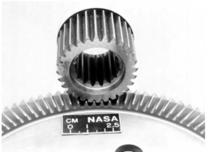
Face gear test hardware.
