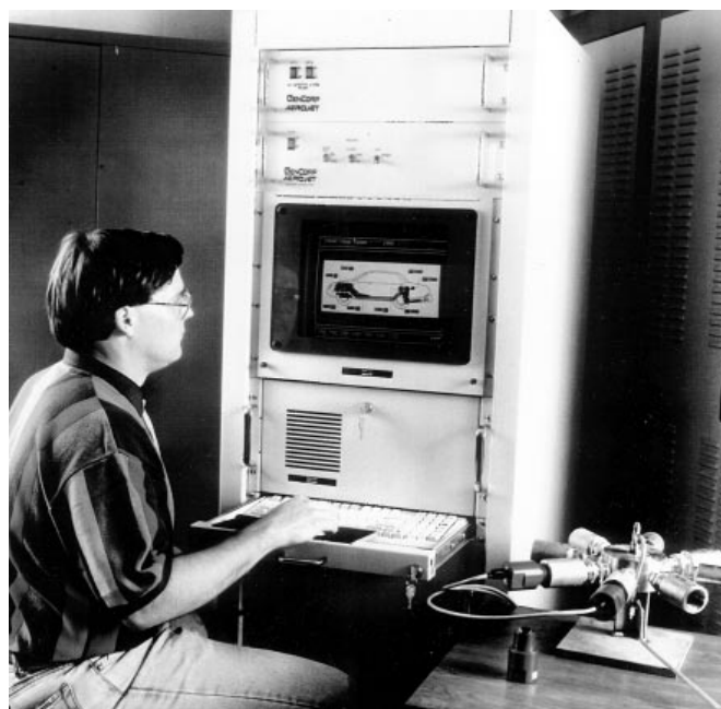
Leak-monitoring system with visual display of leak location.
