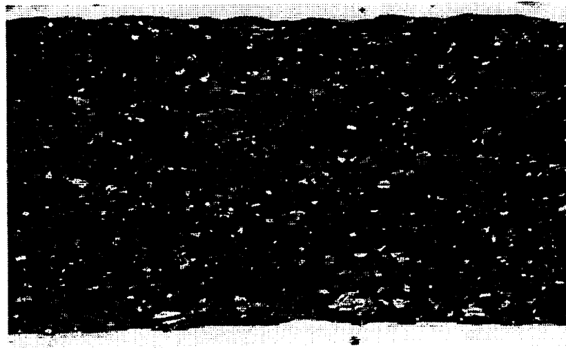
Figure 7.15: As-rolled microstructure of sample IM-4 pack rolled using a \text{CaF}_2 parting agent. The rolling direction is horizontal, and the thickness direction is vertical. (160x)
