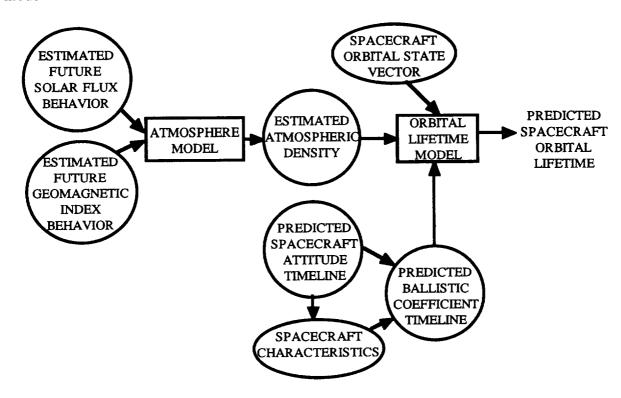
Figure 5-1. MSFC Spacecraft Orbital Lifetime Prediction Model Block Diagram<sup>1,14</sup>.
