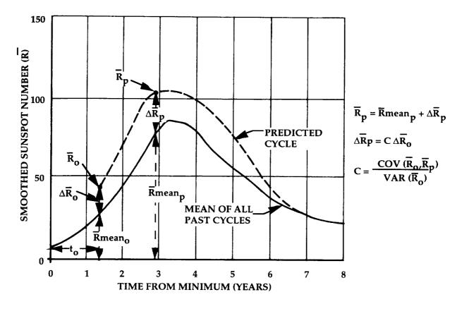
Figure 2-1. Modified McNish-Lincoln Linear Regression Method.
