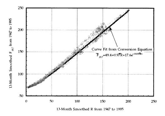
Figure 3-1.  $\overline{R}$  versus  $\overline{F}_{10.7}$  with Curve Fit from Conversion Equation.
