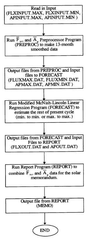
Figure 4-1. MSFC Lagrangian Linear Regression Technique Block Diagram.
