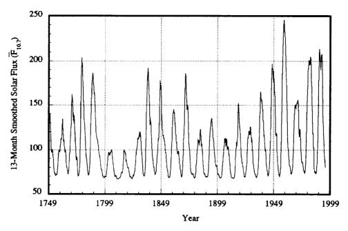
Figure 3-2. 13-Month Smoothed (Converted and Observed) Solar Flux ( $\overline{F}_{10.7}$ ).
