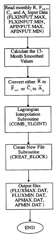
Figure 4-2.  $\overline{F}_{10.7}$  and  $\overline{A}_p$  Preprocessor Computer Program Block Diagram.
