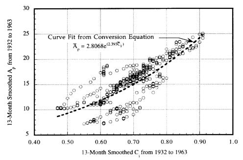
Figure 3-3.  $\overline{C}_i$  versus  $\overline{A}_p$  with Curve Fit from Conversion Equation.
