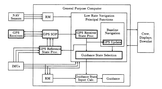
Figure 4.1: Architecture for integrating GPS into navigation subsystem.
