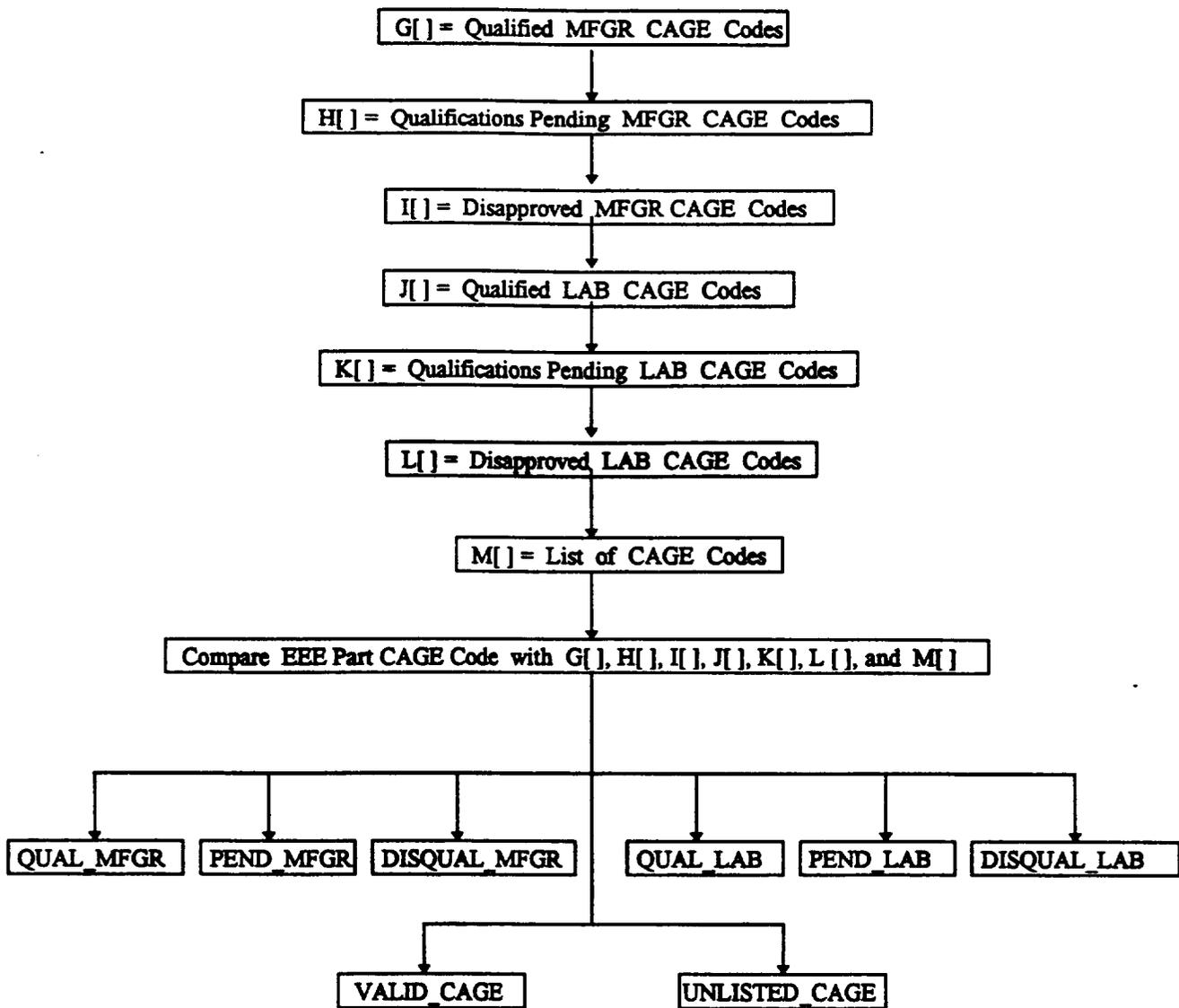
**Figure 5. Flowchart for Screening EEE Parts by Cage Code**
