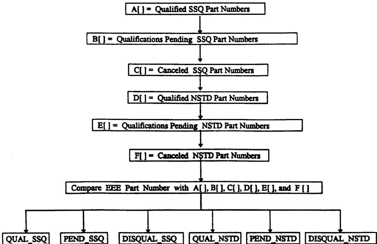
**Figure 4. Flowchart for Screening EEE Parts by Part Number**
