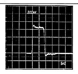
FIG. 5. A high-frequency timing diagram of the measured output voltage of the ORTD when irradiated with a 250 fs, 1.3 μm optical pulse. The frequency response is limited bias elements associated with the RF bias tee. These measurements were performed at the University of Texas microelectronics center.
