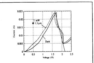
FIG. 3. Room-temperature current-voltage characteristics for the 60  $\mu$ m ORTD under dark and illuminated conditions at a wavelength of 1.3  $\mu$ m.
