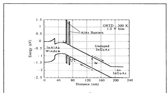
Fig. 2. Computed energy band diagram<sup>5</sup> for the optically switched resonant-tunneling diode. Under bias, electron-hole pairs created within the undoped InGaAs layer screen the electric field present within this layer.
