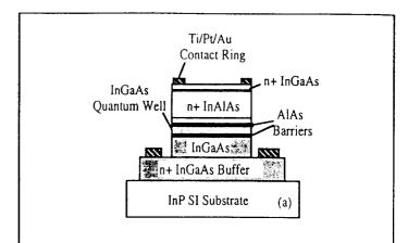
Fig. 1 Schematic cross-sectional diagram for the optically switched resonant-tunneling diode. The epitaxial layers are grown by molecular beam epitaxy within the material science laboratory of Texas Instruments.
