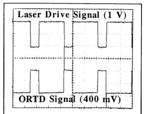
FIG. 4. A low-frequency (1 KHz) timing diagram of the measured output voltage of the ORTD together with the input laser drive signal. The bias conditions for this measurement are 2.1 V through a 100 W resistor.
