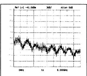
Fig. 6. The measured small-signal frequency response of the 20  $\mu m$  ORTD when illuminated with a 250 fs, 1.3  $\mu m$  impulse signal. These measurements were performed at the University of Texas microelectronic center.
