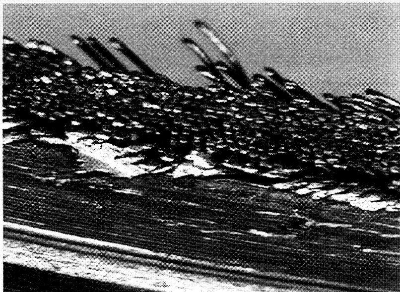
Figure 34.—Outer bristles of brush seal bent axially after testing in LH 2 . Configuration 9.
