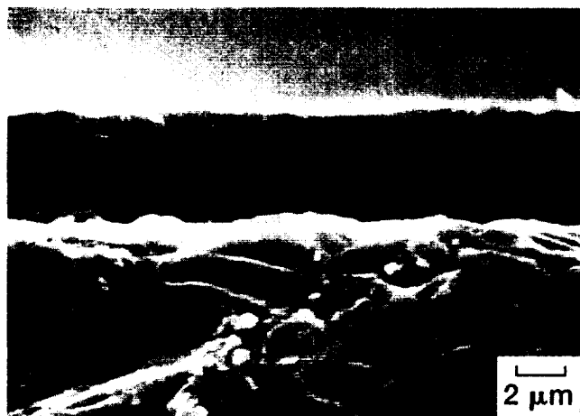
Fig. 3. SEM micrograph showing the oxide scale thickness for two CVD SiC coupons oxidized for 100 h at 1300°C in dry flowing oxygen. The sample on the left was oxidized in an alumina reaction tube and the sample on the right was oxidized in a fused quartz reaction tube.
