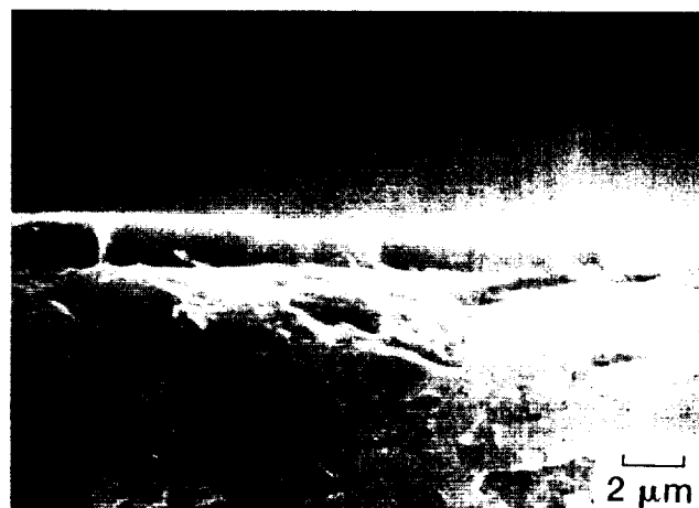
Fig. 3. SEM micrograph showing the oxide scale thickness for two CVD SiC coupons oxidized for 100 h at 1300°C in dry flowing oxygen. The sample on the left was oxidized in an alumina reaction tube and the sample on the right was oxidized in a fused quartz reaction tube.
