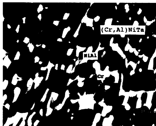
Fig. 10. TEM photomicrograph of an arc-melted NiAl–(Cr, Al)NiTa–Cr eutectic.
