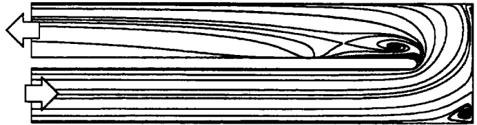
Figure 4. Symmetry plane streamlines for Reynolds number of 17,000 and aspect ratio of 0.5.
