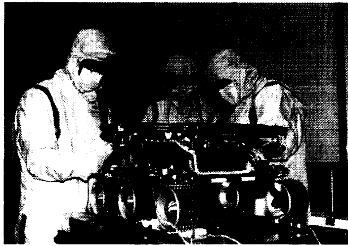
Figure 6.—Sojourner microover during assembly at JPL with WAE visible (middle wheel).
