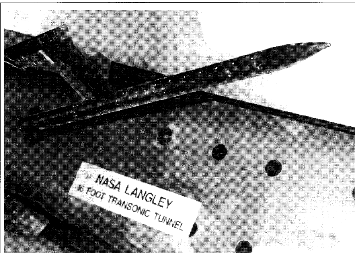
Figure 49. ACT missile model installed in the Langley 16-Foot Transonic Tunnel.
