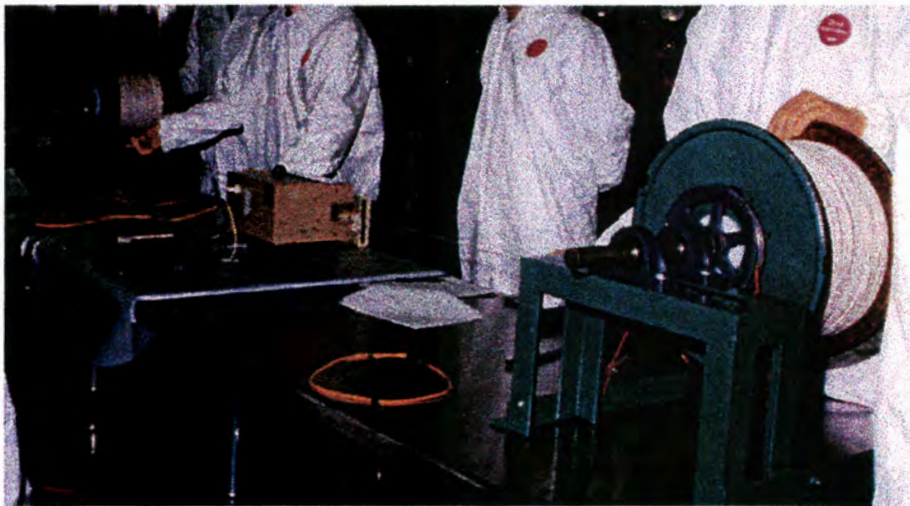
Figure 3.2-25 — Spark Test Set-up
