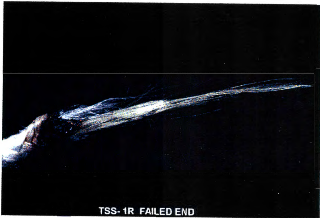
Figure 3.2-4 — Failed End of Flight Tether
