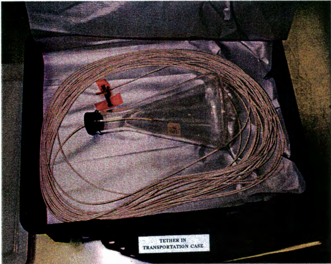
Transporting Failed End of Tether Figure 3.2-3
