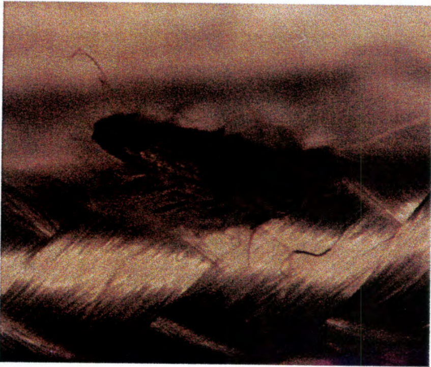
Figure 3.2-12 — Contaminant Particle in Tether
