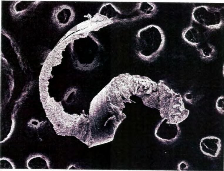
Figure 3.3-11 - SEM image of LTCM Metallic Debris (~1mm Size)
