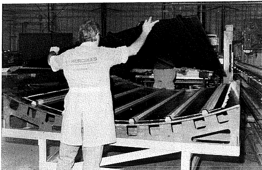
Figure 3-47. Locating Stringers with IML Cauls
