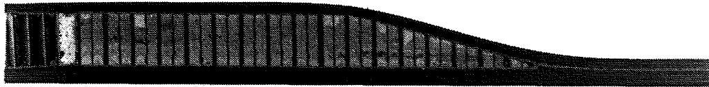
Figure 4-23. Longitudinal Panel Splice Core Close-out Manufacturing Demonstration (Chamfered Foam Filled Honeycomb with Fiberglass/Epoxy Overwrap)
