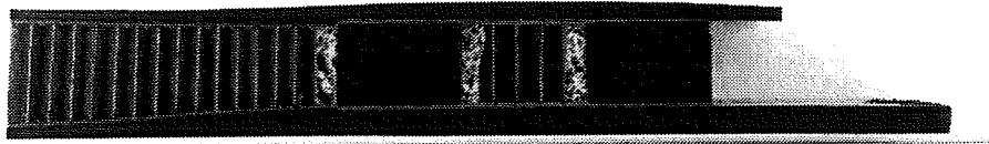
Figure 4-21. Longitudinal Panel Splice Core Close-out Manufacturing Demonstration (Solid Carbon/Epoxy Laminate and Honeycomb with Fiberglass/Epoxy Caps).
