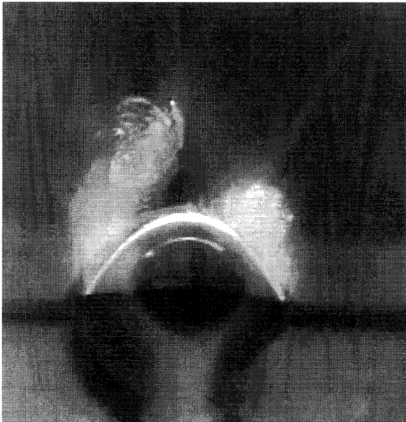
Figure 44. Cross-flow sketch and flow visualization at \alpha = 40^\circ for 1/4 length .3 short ogive strake in front position at \phi_S = 90^\circ with full configuration. View is downstream.
