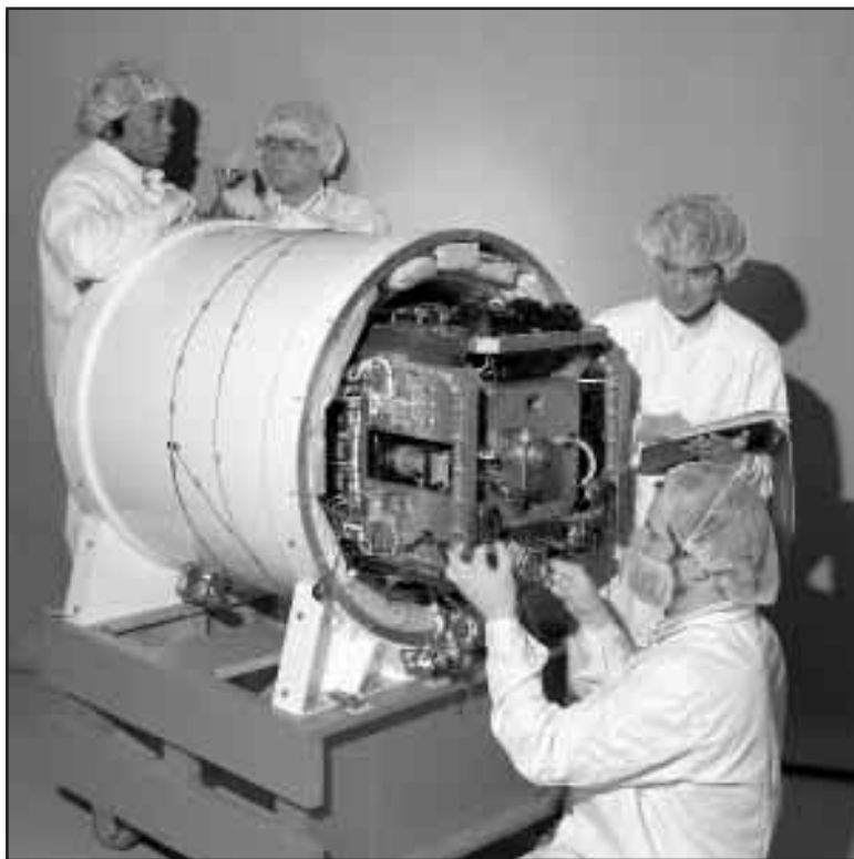
Members of the Lewis-based IDGE team assemble the flight unit. One of the IDGE 35-mm cameras and the Space Acceleration Measurement System (SAMS) sensor head are visible. IDGE is fully operable by remote control from Earth—a feature that contributed to its remarkable success on STS-62 and STS-75.
