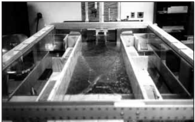
Hydraulic analog model of an ejector-mixer nozzle.
