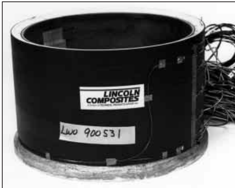
VCAP compressor case after thermal/pressure rig testing at AlliedSignal Engines.
