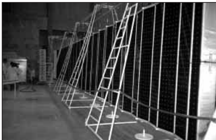
Left: MCSA deployment test in Russia. Right: Comparison of NASA Lewis' electrical performance prediction with on-orbit measurements made by RSC-Energia for a segment of the MCSA known as "GS10."
