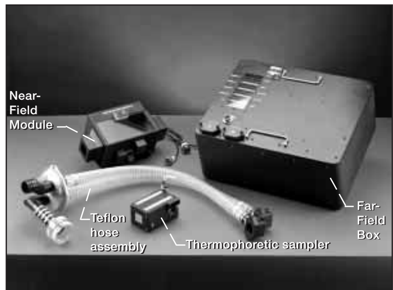
Comparative Soot Diagnostics (CSD) hardware. The Far-Field Box contains space station and space shuttle smoke detectors. The Near-Field Module, which is placed in the Glovebox facility, contains the combustible samples.
