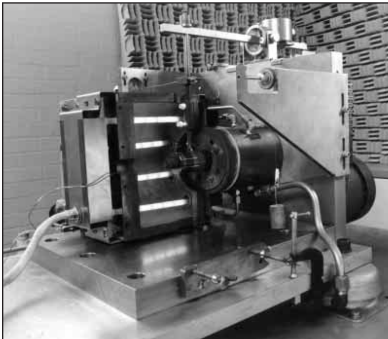
NASA Lewis brush seal tuft tester in operation with half of the furnace shell removed.
