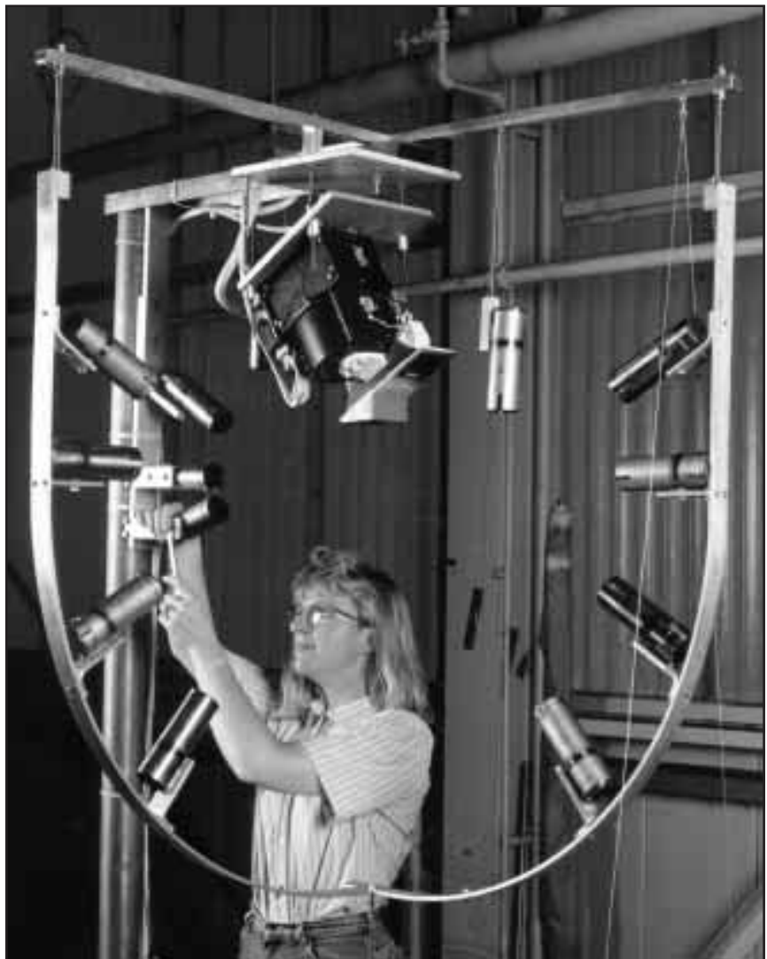
Setting up a pulsed plasma thruster impacts test in a specialized electric propulsion testbed.
