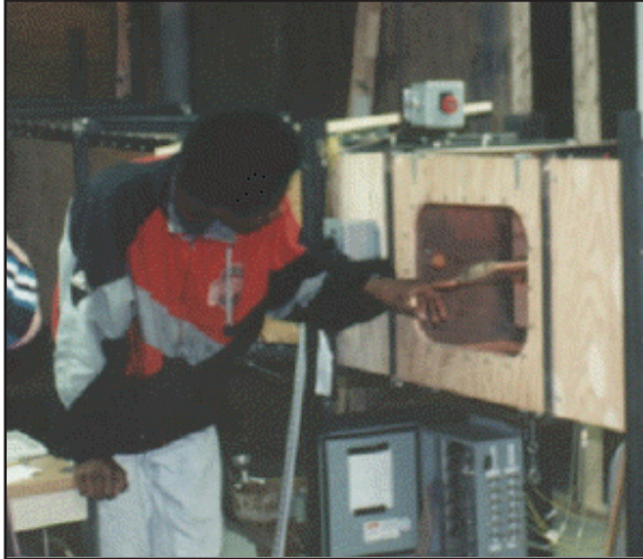
Students at General Benjamin O. Davis Aviation High School test an airfoil in the school's educational wind tunnel.
