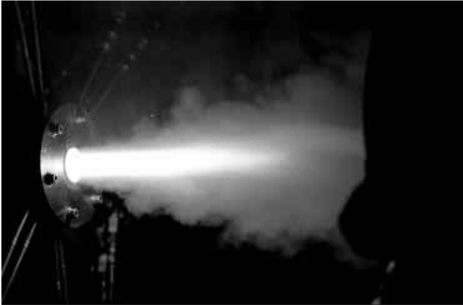
Gelled propellant engine test: 55-wt % RP-1/Al.
