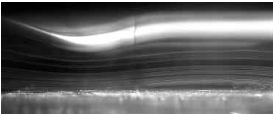
Smoke-wire flow visualization of a separation bubble for a free-stream turbulence level of approximately 0.8 percent.
