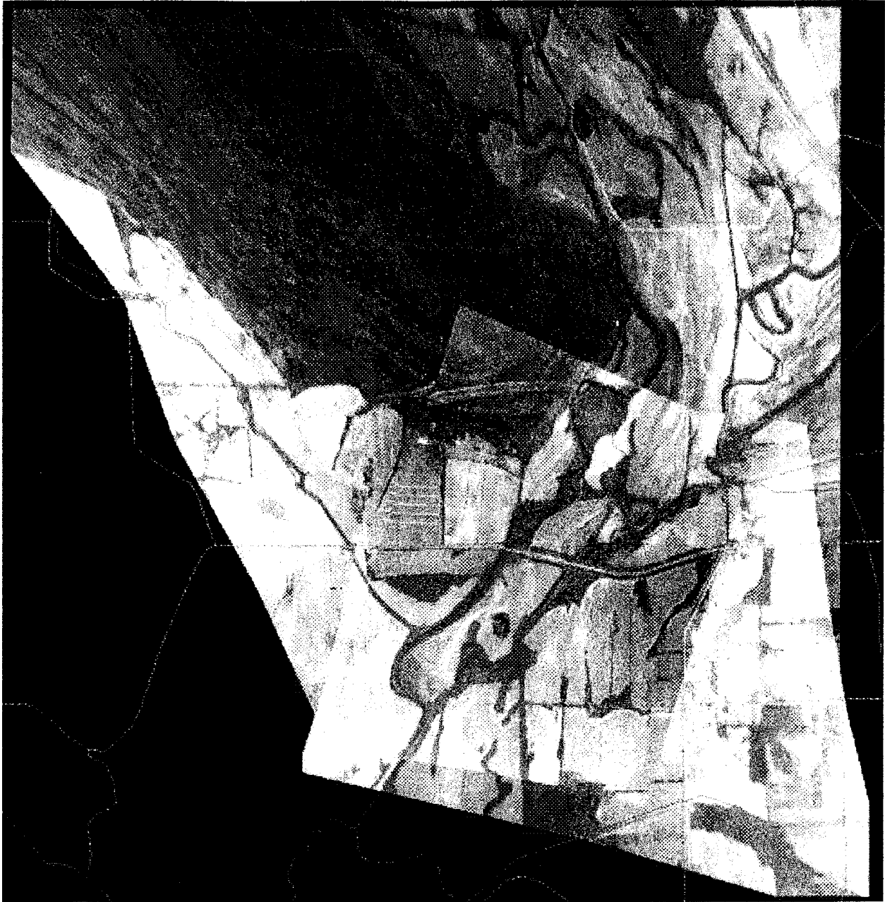
Figure 8. Mosaic image of three aerial photographs taken at different aircraft altitudes, headings, and bank angles.
