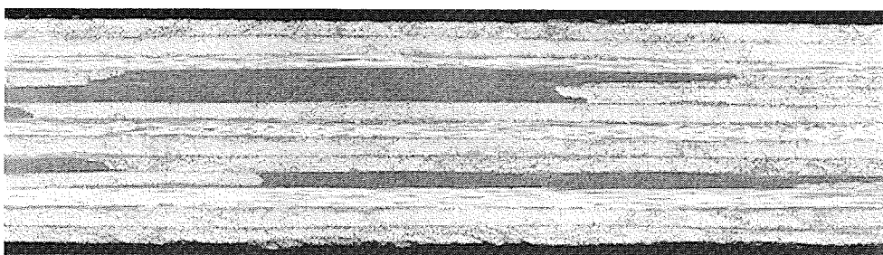
Figure 4-4. Microstructure of an Intraply Hybrid Laminate Fabricated with the Automated Fiber Placement Process (BCA Head).
