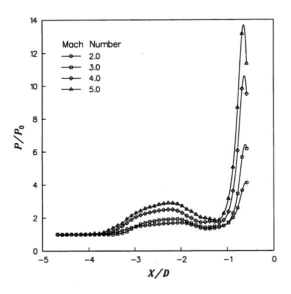
Figure 46 Centerline Static Pressures
