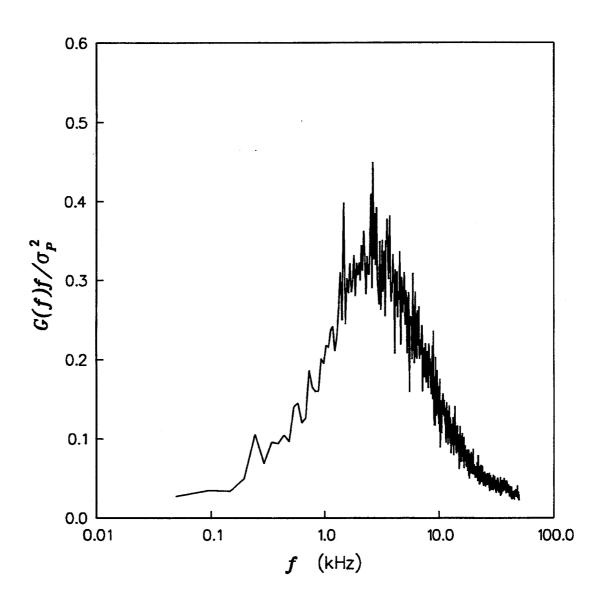
Figure 25 Mach 3.0 Incoming Boundary Layer Normalized Power Spectral Density
