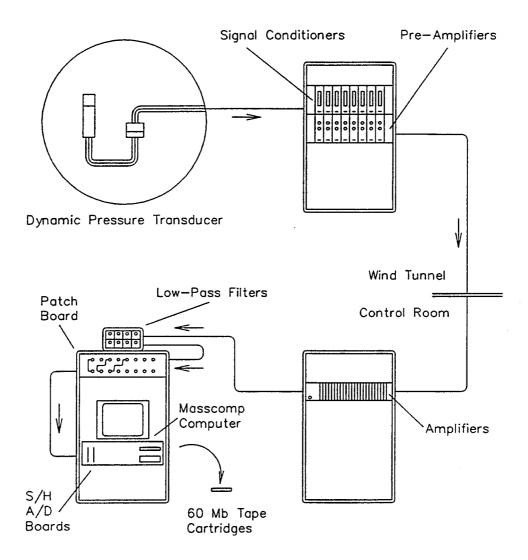
Figure 12 Dynamic Pressure Measurement Data Acquisition System
