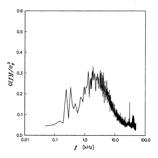
Figure 27 Mach 5.0 Incoming Boundary Layer Normalized Power Spectral Density
