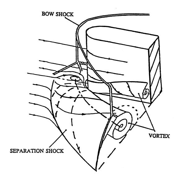
Figure 1 Blunt Fin Induced Shock Wave Turbulent Boundary Layer Interaction
