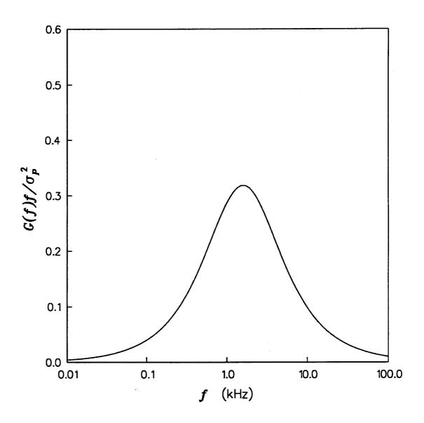
Figure 33 Theoretical Normalized Power Spectral Density Function for all Mach Numbers,  $\Omega = 0.1 \text{ ms}$
