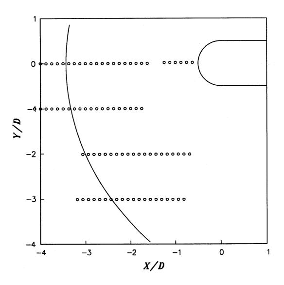
Figure 55 Mach 5.0 Dynamic Pressure Transducer Measurement Locations
