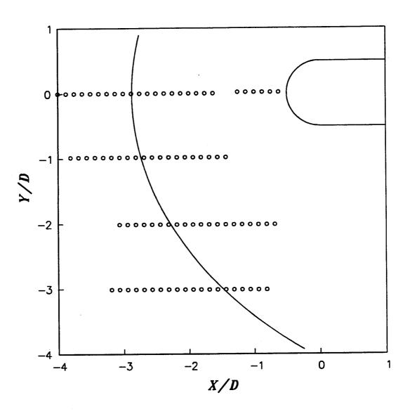
Figure 53 Mach 3.0 Dynamic Pressure Transducer Measurement Locations
