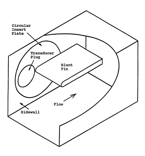
Figure 3 Test Section
