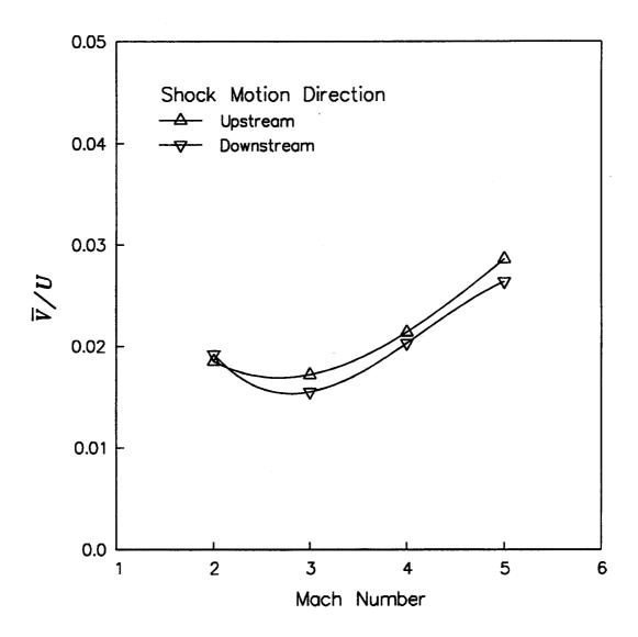
Figure 88 Centerline Mean Shock Velocity
