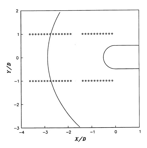
Figure 111 Mach 3.0 Dynamic Pressure Transducer Locations for Latteral Correlation Measurements
