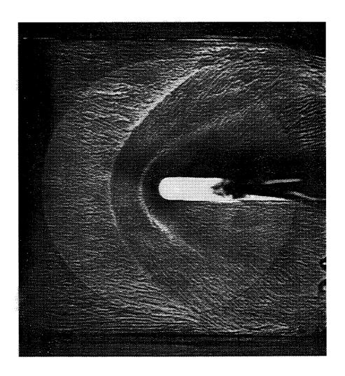
Figure 39 Mach 4.0 Interaction Surface Flow Visualization
