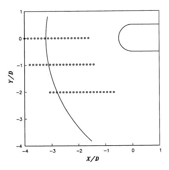
Figure 54 Mach 4.0 Dynamic Pressure Transducer Measurement Locations
