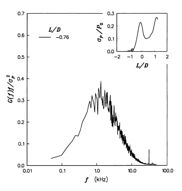
Figure 89 Mach 3.0 Centerline Power Spectra (1 of 5)
