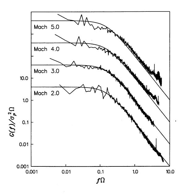
Figure 32 Comparison of Incoming Boundary Layer Power Spectral Density Functions with Theory
