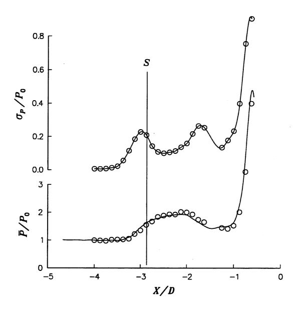
Figure 66 Mach 3.0 Centerline Comparison of Mean Pressures and Standard Deviations
