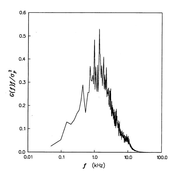
Figure 17 Example of a Normalized Power Spectral Density Function
