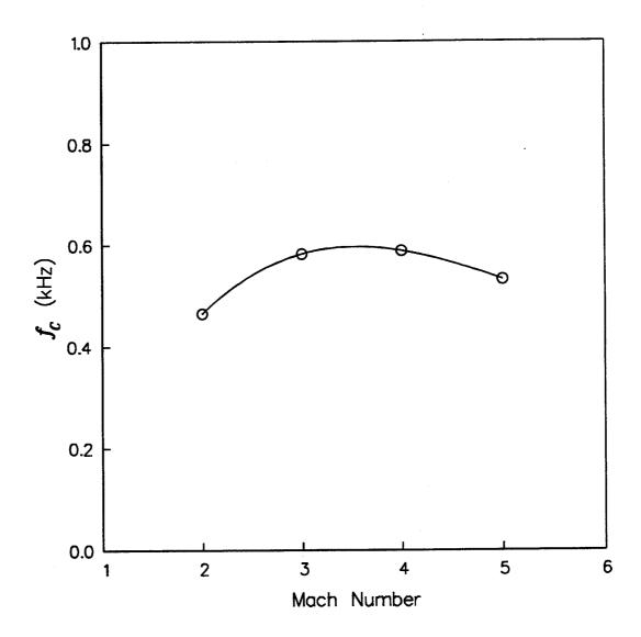
Figure 85 Centerline Maximum Zero-Crossing Frequency
