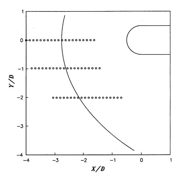
Figure 52 Mach 2.0 Dynamic Pressure Transducer Measurement Locations
