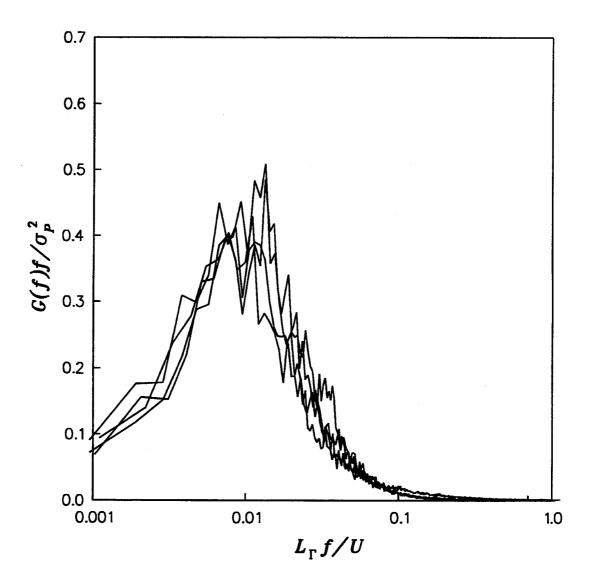
Figure 97 Centerline Power Spectra Comparison Mach Numbers 2.0, 3.0, 4.0, and 5.0
