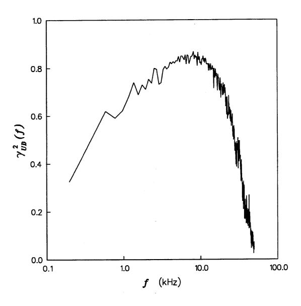
Figure 113 Mach 3.0 Incoming Boundary Layer Longitudinal Coherence Function
