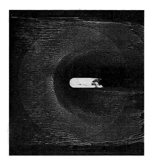
Figure 37 Mach 2.0 Interaction Surface Flow Visualization
