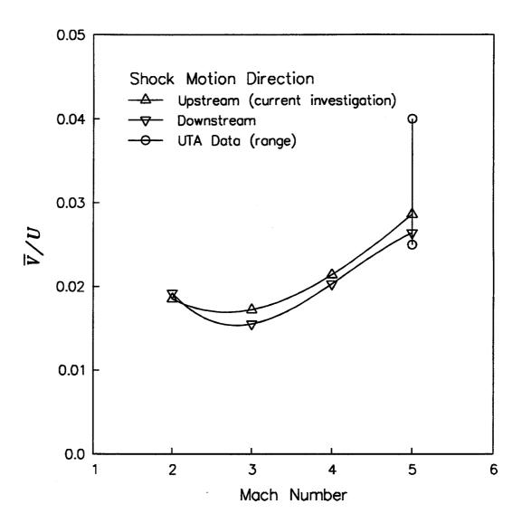
Figure 105 Centerline Mean Shock Velocity Comparison
