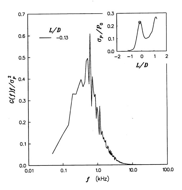
Figure 91 Mach 3.0 Centerline Power Spectra (3 of 5)
