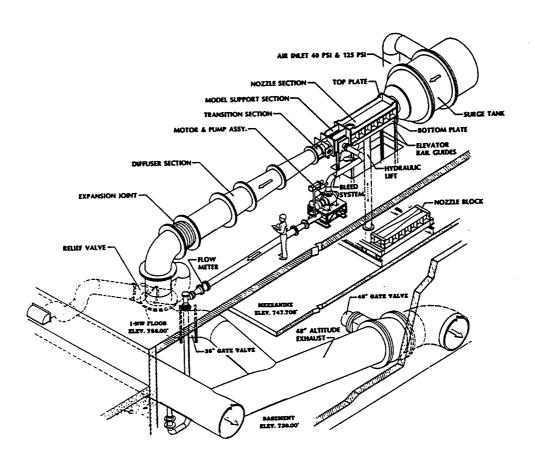
Figure 2 1x1 Supersonic Wind Tunnel
