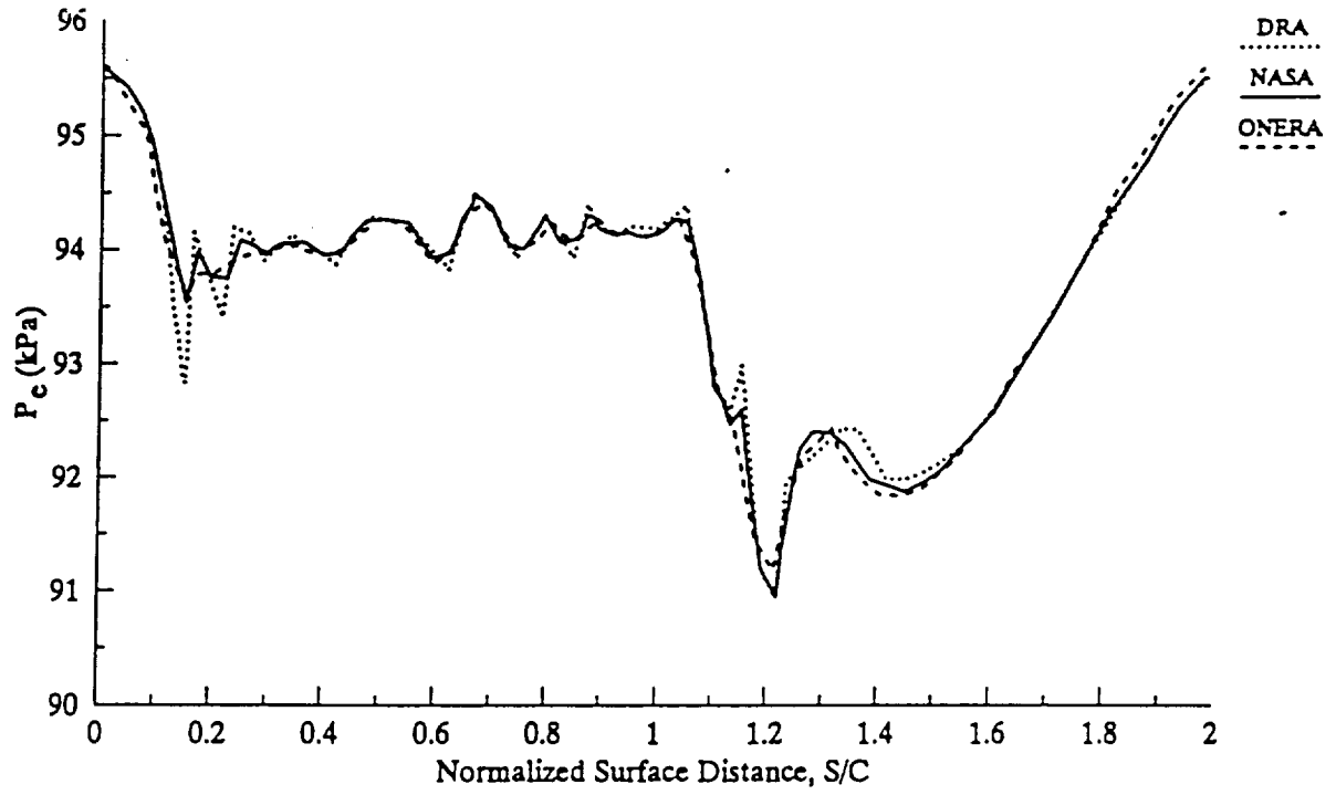
Figure 22 - 15 min Rime Iced Cylinder (Smooth Case)
