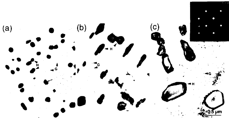
FIG. 14. TEM BF images from homogenized and air-cooled NiAl-1.0 at. % Hf samples after aging for (a) 1, (b) 100, and (c) 500 h at 1300 K. A [001] zone axis microdiffraction pattern of one of the large Heusler precipitates in (c) is included.
