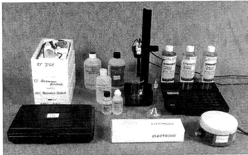
Figure 12.—Ion-specific electrode setup.
