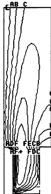
Figure 9. Azimuthal Velocity distribution (m/s) for the 0.102 T, 1000 A case.
