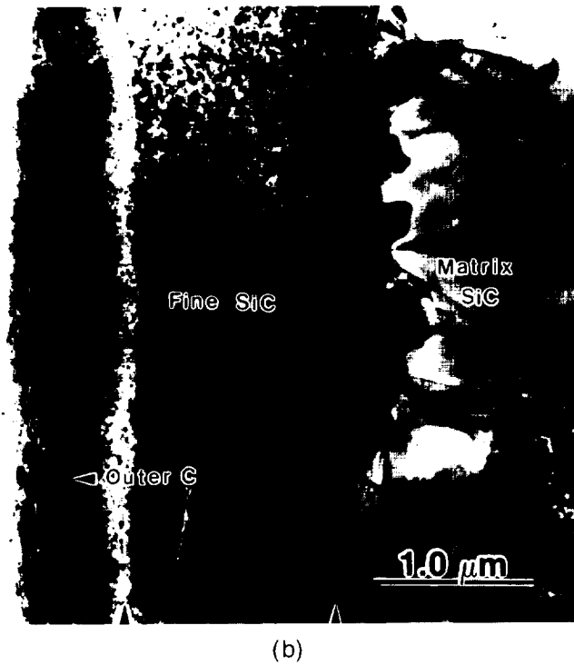
FIG. 6. Bright-field TEM micrographs of the fiber/matrix interface. The SiC fiber/inner carbon-rich layer (a) and outer carbon-rich layer/matrix SiC regions are shown in (b).
