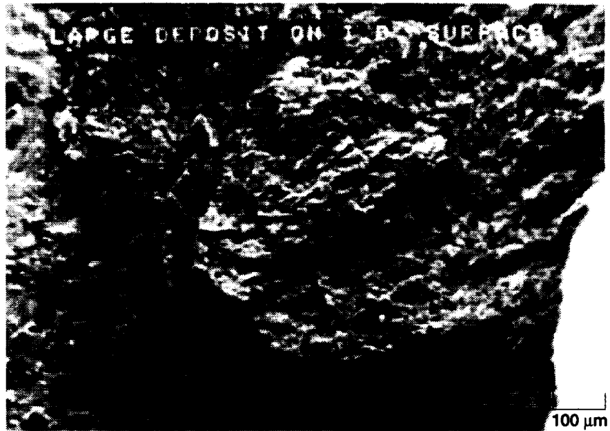
Figure 17.—Carbon deposit adjacent to failure site. Fractured and flake-like appearance.
