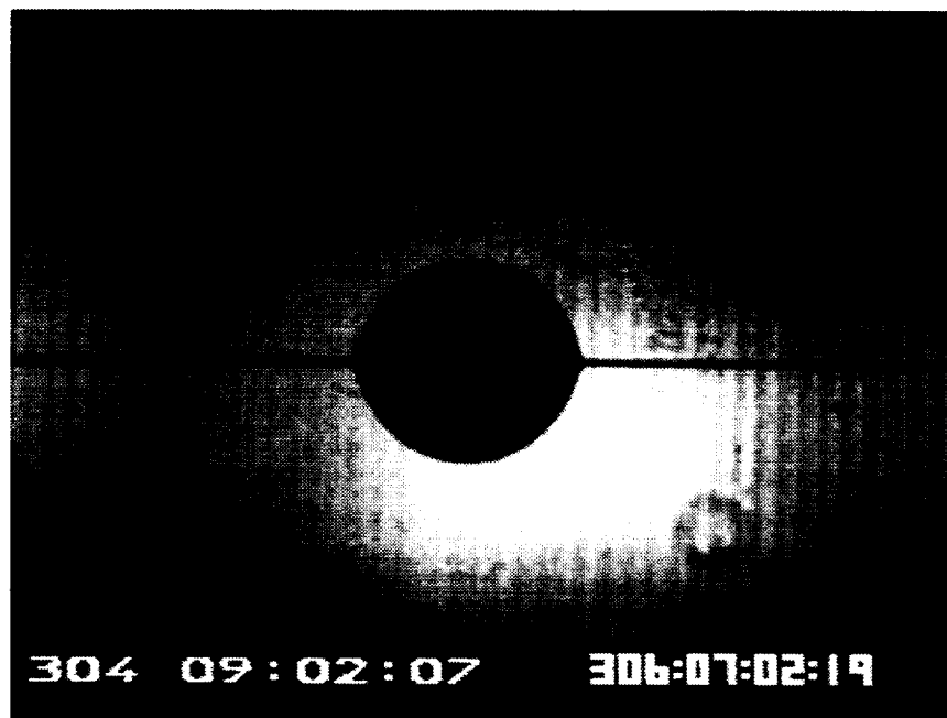
8 mm diameter fluid droplet in microgravity suspended on a fiber support.
