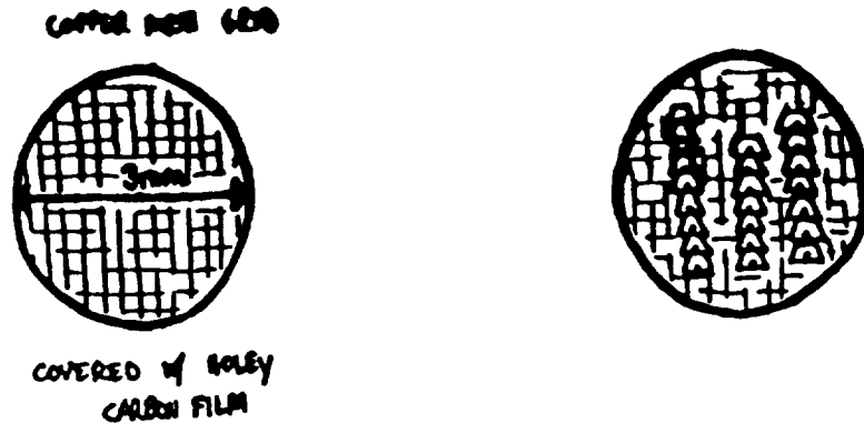
Figure 1.2 Three steps in preparing samples for TEM analysis. 1) Grains are embedded in an epoxy block. 2) The epoxy block is fashioned with razor blades and glass knives until a small trapezoidal face is formed with the grains directly below the epoxy surface. Thin sections are then cut with a diamond knife. 3) Thin sections are then mounted on copper grids. Note that all sections containing sample is the ideal case.
