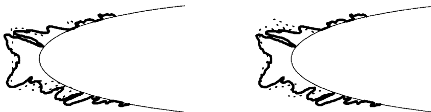
(a) Scaling Using Ruff (Mod) Method. (b) Scaling Using Constant- We Method.
