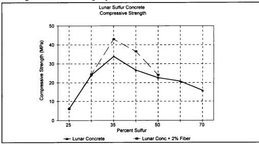
Compressive and tensile strengths of sulfur concrete obtained in the exceed those for hydraulic cement concretes. The maximum compressive strength of non-reinforced sulfur concrete was found to be 33.8 MPa for a 35% sulfur content by weight. While the maximum strength for the same sulfur concrete with the addition of 2% by weight Aluminum fibers was found to be 45.5 MPa.
