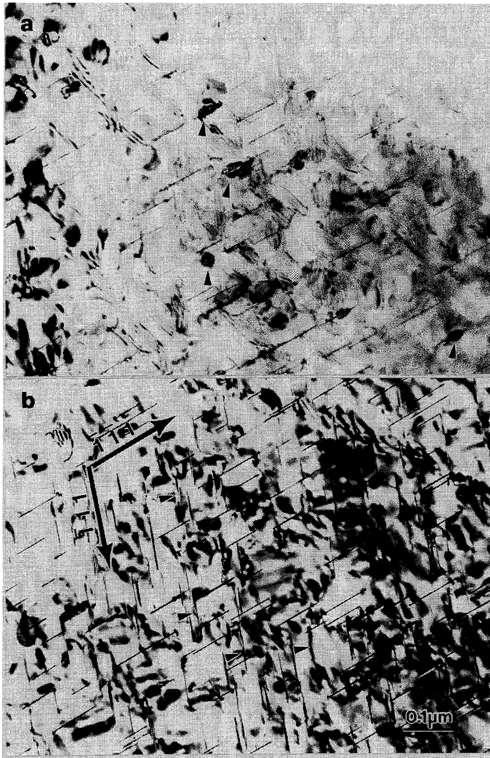
Figure 15. TEM BF images of 2195, aged for 15h at 149°C, DSC scanned up to 300°C and liquid N 2 quenched. (a) g=[-111] , near B=[101] ; (b) B=[101] .
