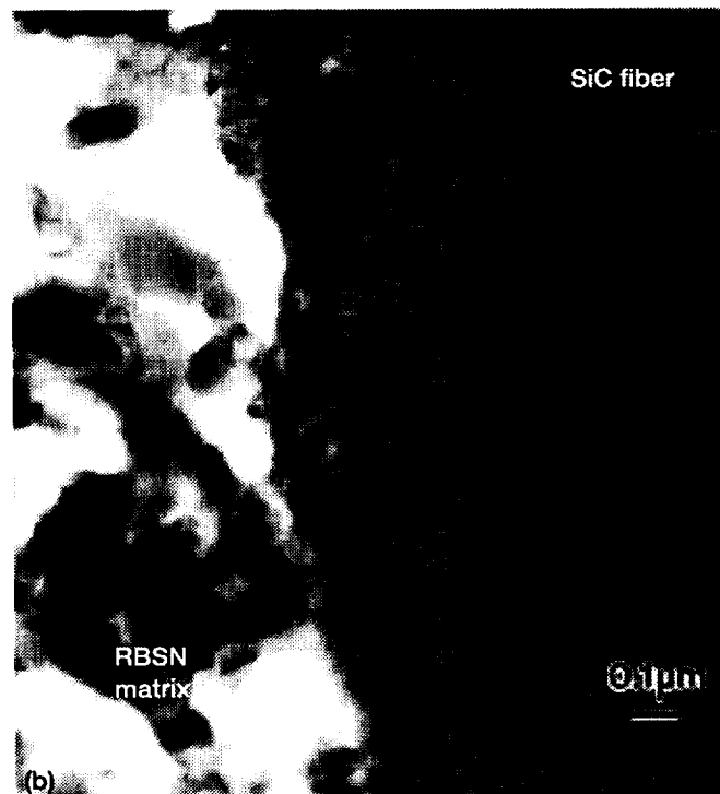
Figure 8.—TEM micrographs of the PBN/Si-PBN coated Hi-Nicalon/RBSN tow composite nitrided at 1400 °C in N 2 for 4 hr showing reaction between the fiber and RBSN matrix. (a) PBN/Si-rich PBN and RBSN interface. (b) Region of the uncoated fiber showing reaction with iron and nickel.
