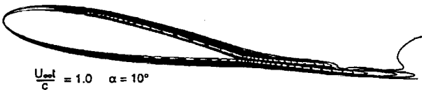
Fig. 7 Vorticity contour plot for the flow near the airfoil at U_{\infty}t/c = 1.0 . Note the residues of the starting vortex at the right-hand side of the computational domain.
