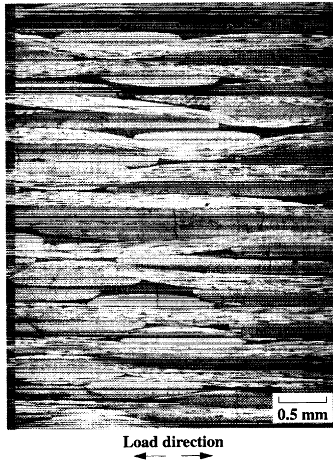
Figure 3.22 Edge view of transverse cracks as observed by microstructural examination of 22 °C (72 °F) specimen with 1% stiffness reduction (view #2; see Figure 2.7): 25x magnification: \sigma_{max} = 379 MPa (55 ksi); N_{interrupt} = 208 ; Specimen PC3_10.
