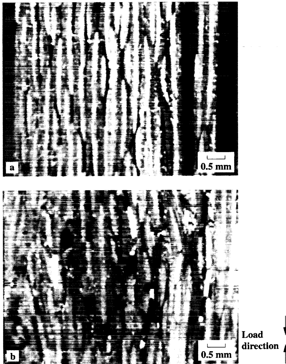
Figure 3.36 Residual compression strength coupon at 22 °C (72 °F) as observed using video images of monitored edge view with 15x magnification. Initial damage state included a delamination induced by the fatigue test. (a) Image taken at -462 MPa (-67 ksi) right before failure. (b) Failure at -483 MPa (-70 ksi): Damage = 0.89E_0 ; Specimen PC3_16c.
