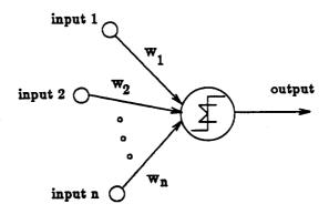
Figure 1: A prototypic ANS unit. Inputs from units 1 through n are summed together along weighted connections, w, to produce an activation value. That activation value is then typically thresholded to produce an output value for the unit.
