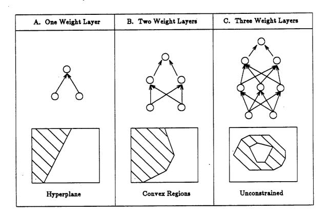
Figure 5: Computable output regions for three different network architectures (after Lippman 1987). 5a: A network composed of one layer of weights is restricted to dividing the output space into two distinct hyperplanes. 5b: A two-layered network may represent functions which map into convex open or closed regions. 5c: A three-layered network given enough hidden units, is unconstrained and has the capacity to represent any arbitrary function.
