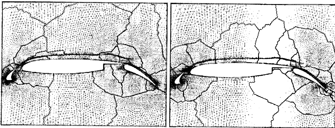
FIG. 9.2. Comparison of Unweighted (Left) and Weighted (Right) 32-Way Partition of Unstructured Mesh for Parallel Computation
