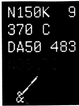
Figure 1. Conflict aircraft callsign displayed in the fourth line of the flight data block.
