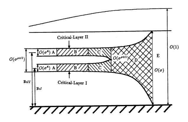
Fig. 2 Nonlinear interaction between the frequency-detuned resonant-triads I and II in an adverse-pressure-gradient boundary layer where  $\rho < 3$ . A, linear stage; B, parametric-resonance stage; C, fully-coupled stage; D, frequency-detuned nonlinear-interaction stage; E, triple-deck stage.
