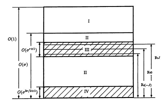
Fig. 1 Multi-layer structure for the non-equilibrium critical-layer analysis of multi-resonant-triads in boundary layers. I, main boundary layer; II, inviscid Tollmien wall layer; III, critical layer; IV, viscous Stokes layer.
