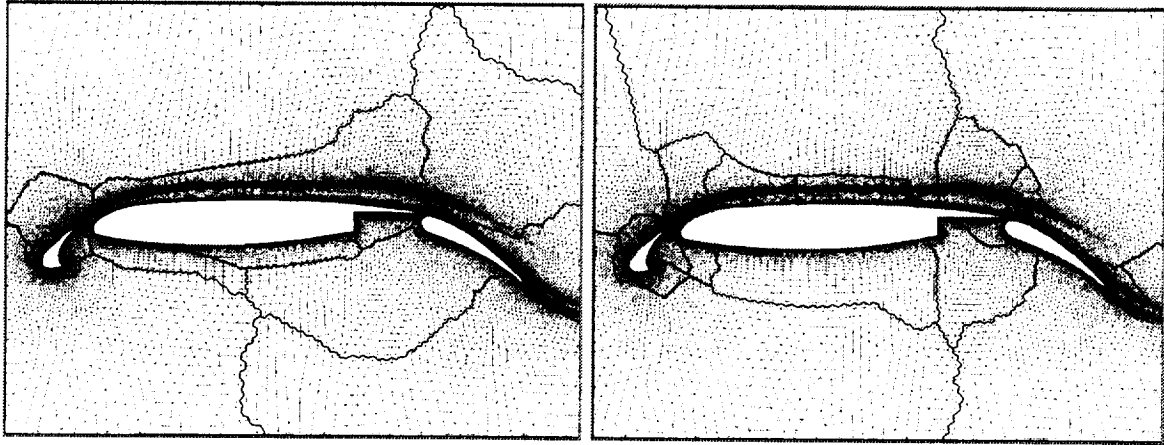
FIG. 5.2. Comparison of Unweighted (above) and Weighted (below) 32-Way Partition of Two-Dimensional Mesh
