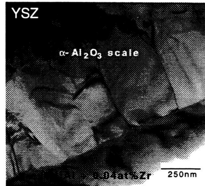
TEM bright field image x-section of the \text{Al}_2\text{O}_3 scale beneath YSZ top coat after 2h at 1200°C
