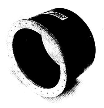
Figure 4-8. Completed Compressor Case
