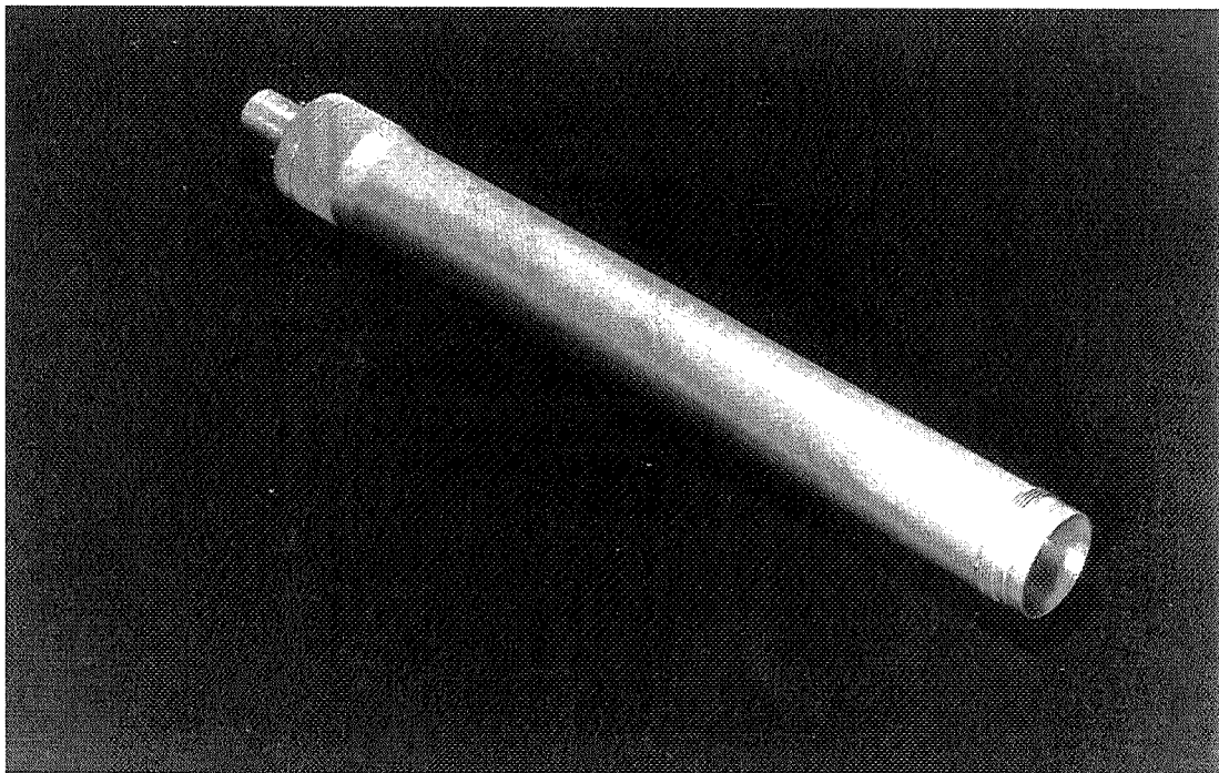
Figure 5. - 4-cm diameter drive tube. This tube has threads near the bottom which allow it to be screwed into another tube section. The tube on the bottom (not shown) has a steel bit formed into the aluminum tube in place of the threads (NASA photo S-71-16526).
