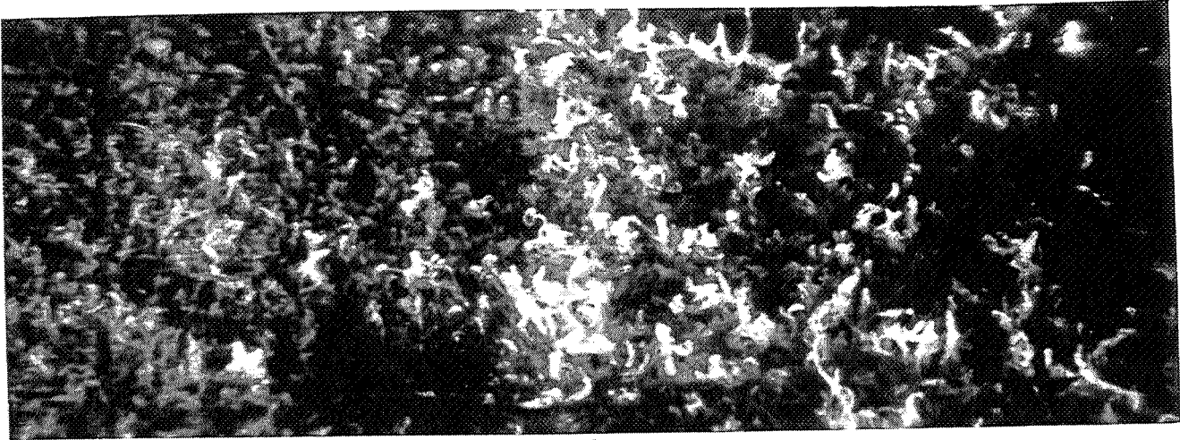
Fig. 1 - A view of an amorphous ice layer, seen at an oblique angle. Needles about 0.1 mm long are seen, with an ice layer containing \sim 10^{20} water molecules/cm 2 .
