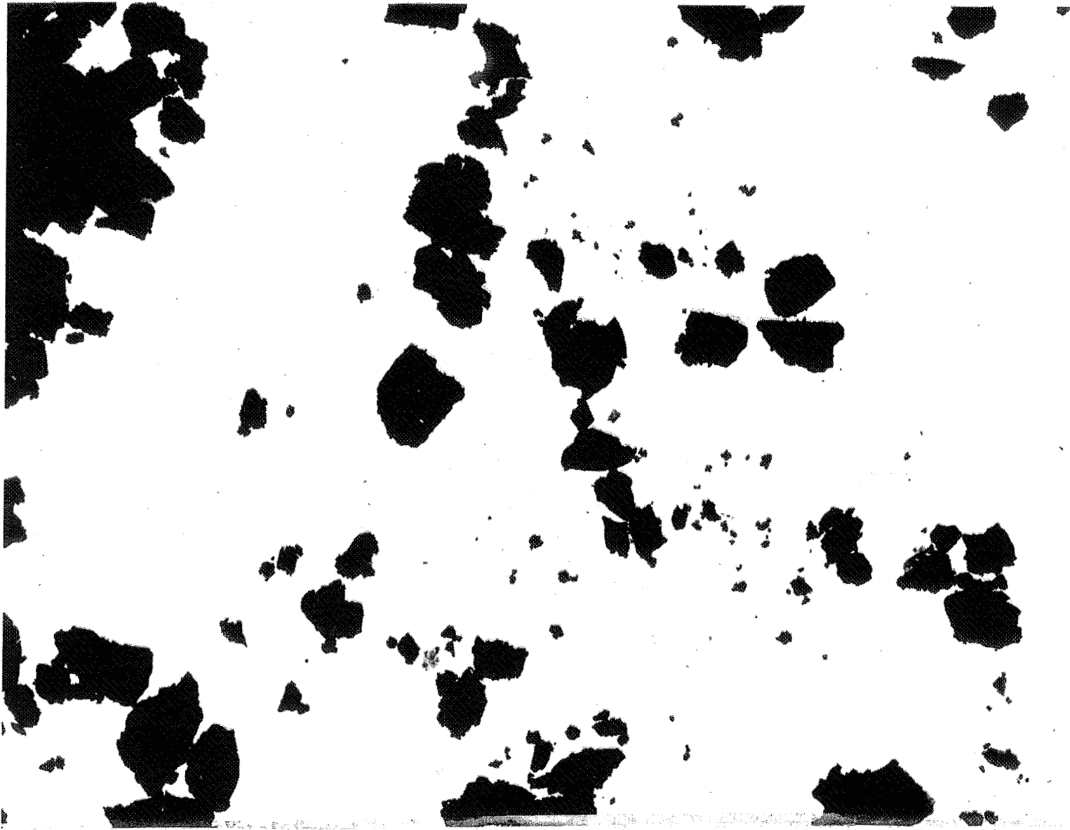
Figure 3.- TEM micrograph of an \alpha -SiC sample; the irregular shape of the grains is evident.
