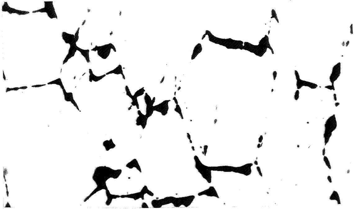
Figure 6.- Polycrystalline ice produced from a water-carbon suspension (soot of ca. 25 nm grain size) with carbon aggregates occupying grain boundaries of ice crystals; polished section in reflected light; horizontal width of image: 0.7 mm
