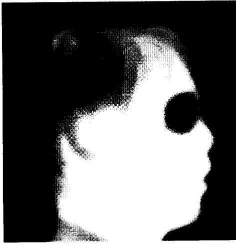
Fig. 10. One frame from a 15- \mu\text{m} QWIP video image of a man's face with NE\Delta T = 30 mK.
