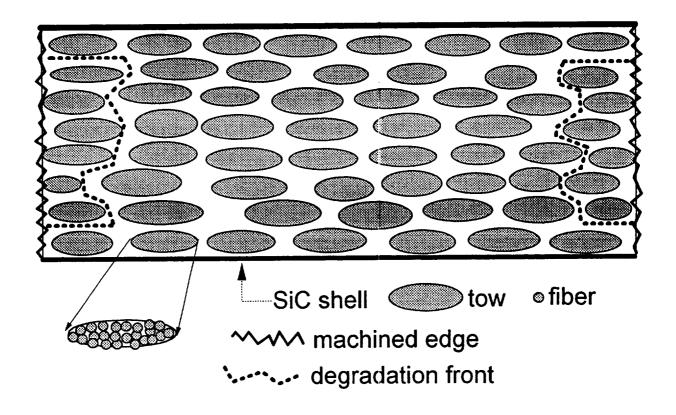
Fig. 1 Schematic diagram illustrating the inward advance of environmental degradation, one tow at a time, expected (and often observed) in SiC-SiC composites.
