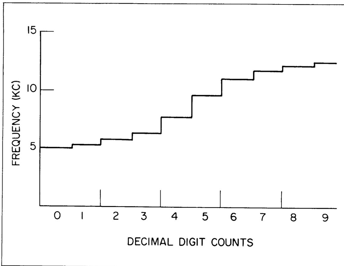
Figure 2 - Telemetering frequency vs counts, 1959 Eta
