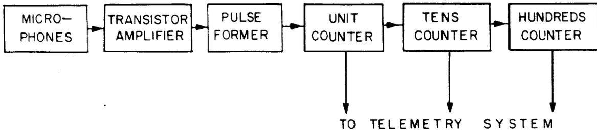
Figure 1 - Block diagram of micrometeorite counter
