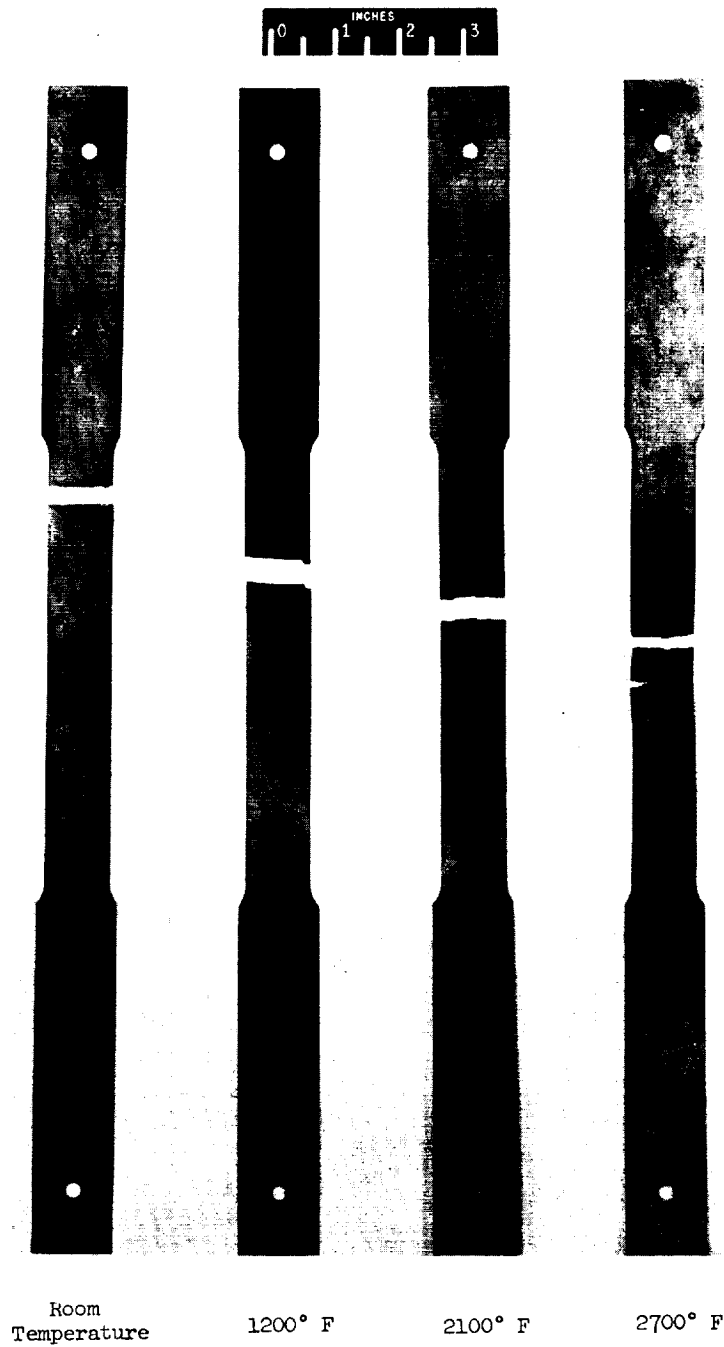
Figure 10.- Examples of fractures obtained at several temperatures in tensile stress-strain tests of W-2 coated Mo-0.5Ti sheet in reprocessed condition. Sheet thickness, 0.010 inch; W-2 coating thickness, 0.001 inch.
