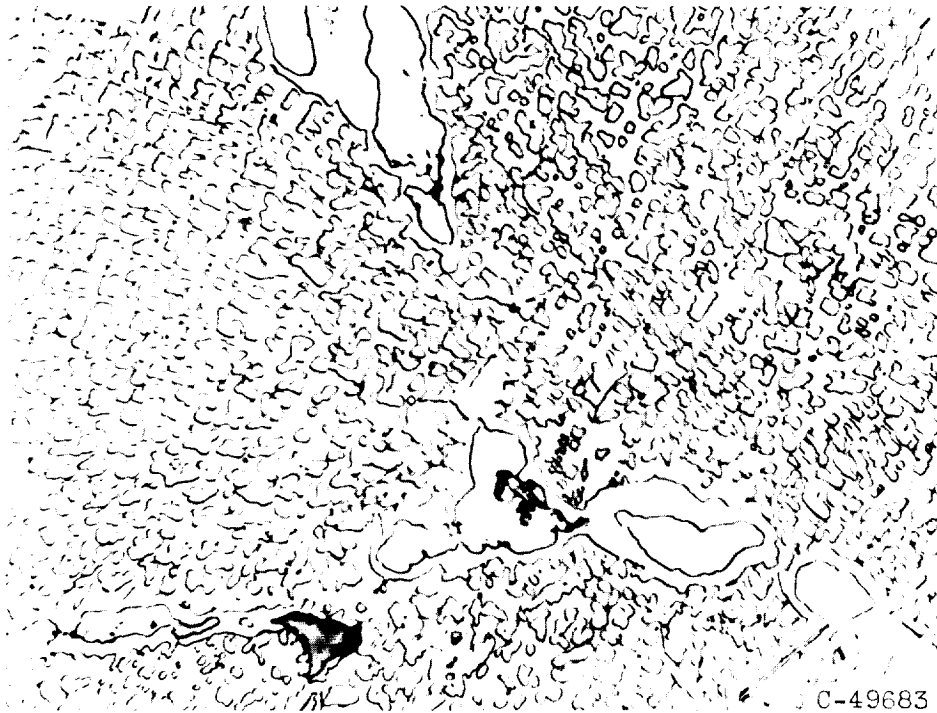
(d) Basic alloy + 1.5 Ti + 0.125 C, heat-treated 16 hours at 2000° F.
