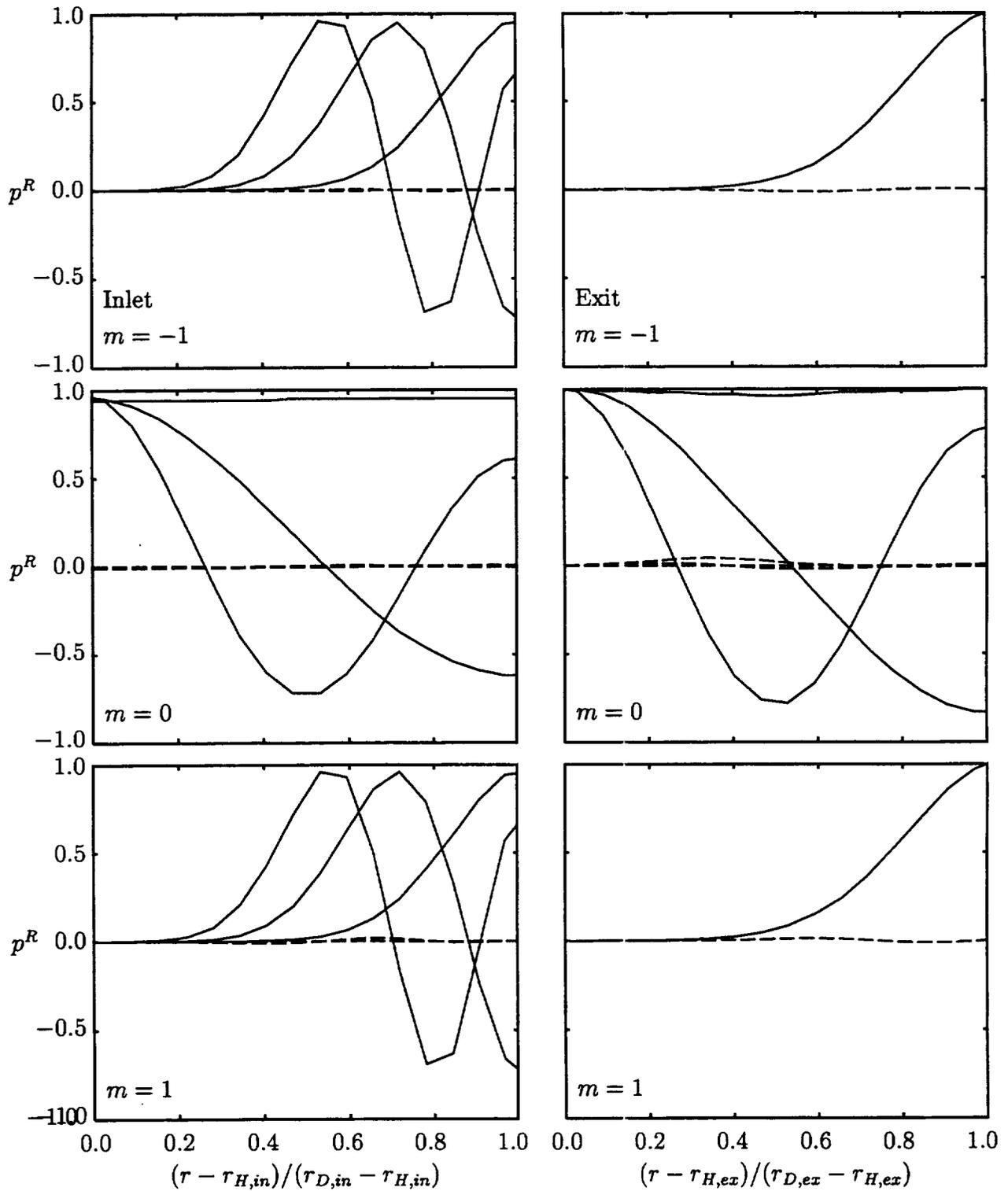
Figure 26: First harmonic, radial pressure modes,  $p_{m\mu}^R(r)$ ,  $m = -1, 0, 1$ ,  $\mu = 0, 1, 2$ , for an acoustic excitation or response, at  $N_D = 0$ , far upstream and for an acoustic response, at  $N_D = 0$ , far downstream of the Rotor 67 fan: (—) in-phase component; (---) out-of-phase component of  $p_{m\mu}^R(r)$ .
