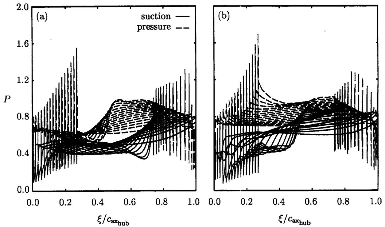
Figure 22: Steady static pressure distributions for the Rotor 67 fan (a) near the peak efficiency point, and (b) near stall.
