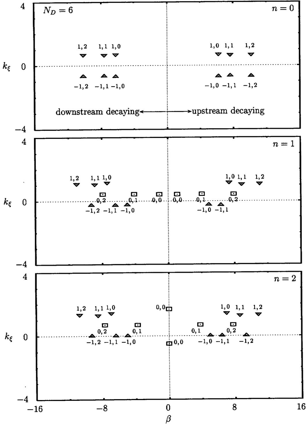
Figure 12: Axial eigenvalues,  $\chi = \beta + ik_\xi$ , at exit for three circumferential ( $m = -1, 0, 1$ ) and three radial ( $\mu = 0, 1, 2$ ) modes of steady ( $n = 0$ ), first-harmonic ( $n = 1$ ) and second-harmonic ( $n = 2$ ) acoustic disturbance in an unsteady flow at  $\omega = 1.0$  and  $N_D = 6$ , through the 3D 10th Standard Cascade.
