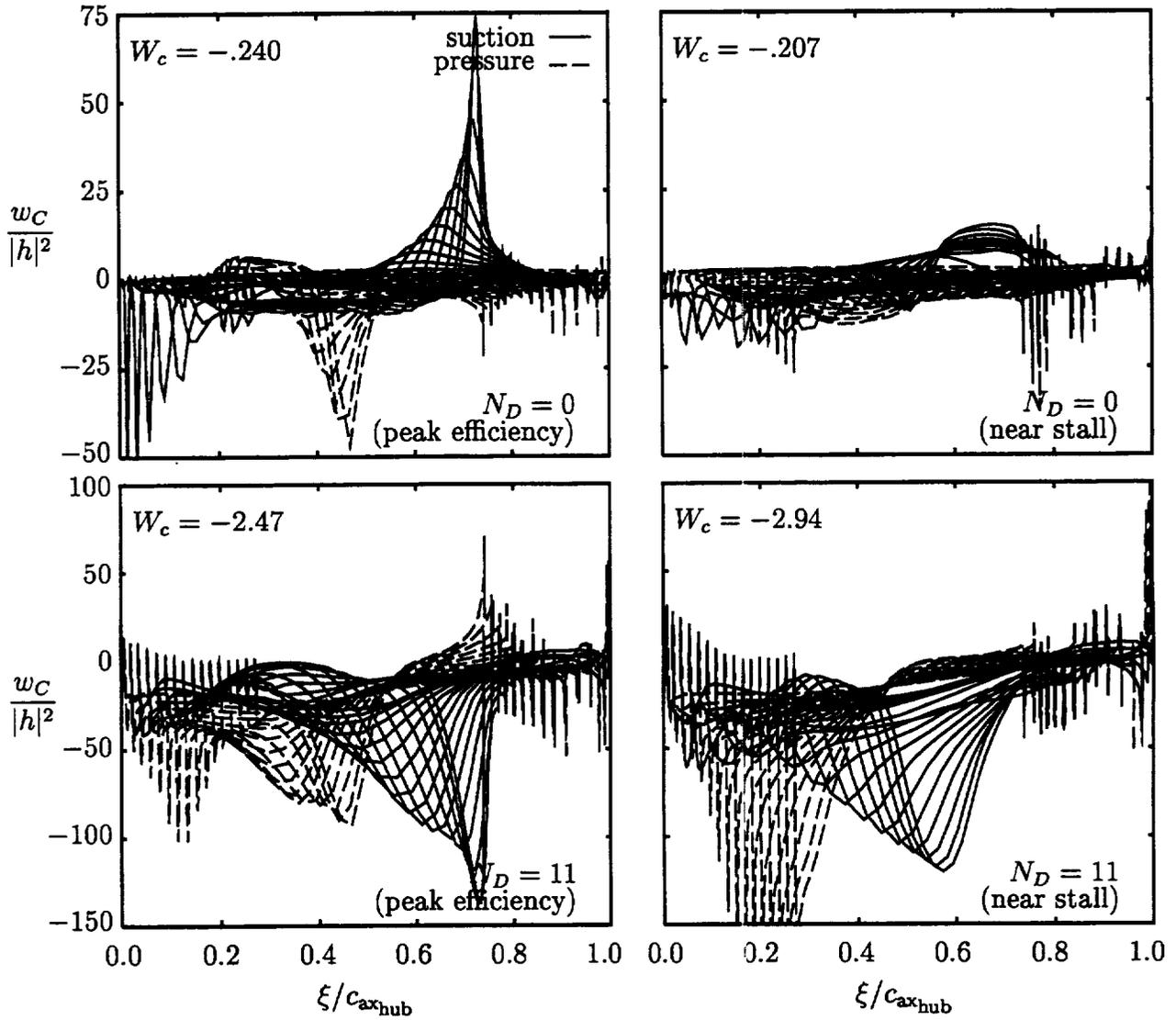
Figure 28: Local work per cycle distributions and global works per cycle for the Rotor 67 fan undergoing pure bending vibrations at  $\omega = 0.54$  and  $\sigma = 0$  and  $180$  deg ( $N_D = 0$  and  $11$ ).
