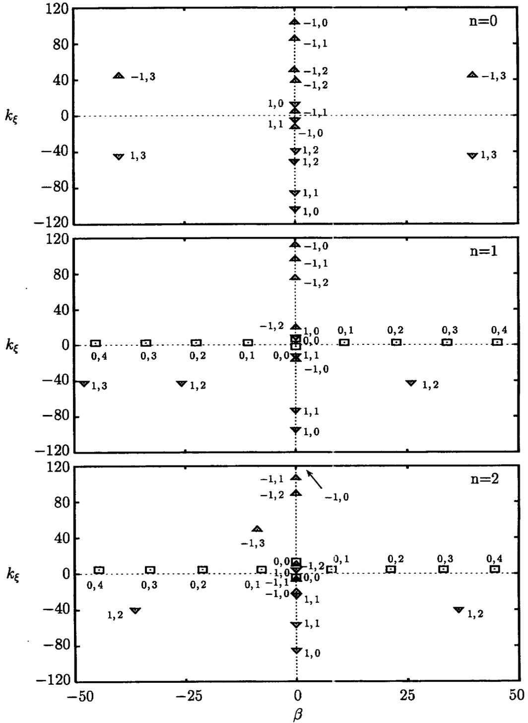
Figure 24: Axial eigenvalues,  $\chi = \beta + i\kappa_\xi$ , at inlet for the time-mean ( $n = 0$ ), and the first ( $n = 1$ ) and second ( $n = 2$ ) temporal harmonics, and three circumferential ( $m = -1, 0, 1$ ) and five radial ( $\mu = 0, 1, 2, 3, 4$ ) modes of acoustic disturbance in the far field of Rotor 67, for an unsteady flow at  $\omega = 0.54$  and  $N_D = 0$ , and a meanflow condition near peak efficiency.
