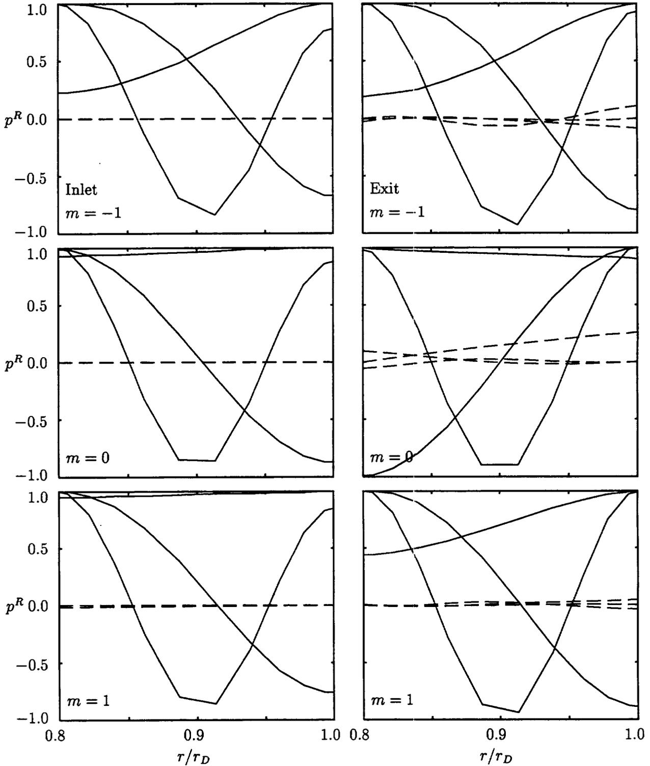
Figure 13: First harmonic, radial, pressure modes,  $p_{m\mu}^R(r)$ ,  $m = -1, 0, 1$ ,  $\mu = 0, 1, 2$ , at inlet and exit due to an acoustic excitation or response, at  $N_D = 6$ , far upstream and for an acoustic response, at  $N_D = 6$ , far downstream of the 3D 10th Standard Cascade: (—) in-phase component; (---) out-of-phase component of  $p_{m\mu}^R(r)$ .
