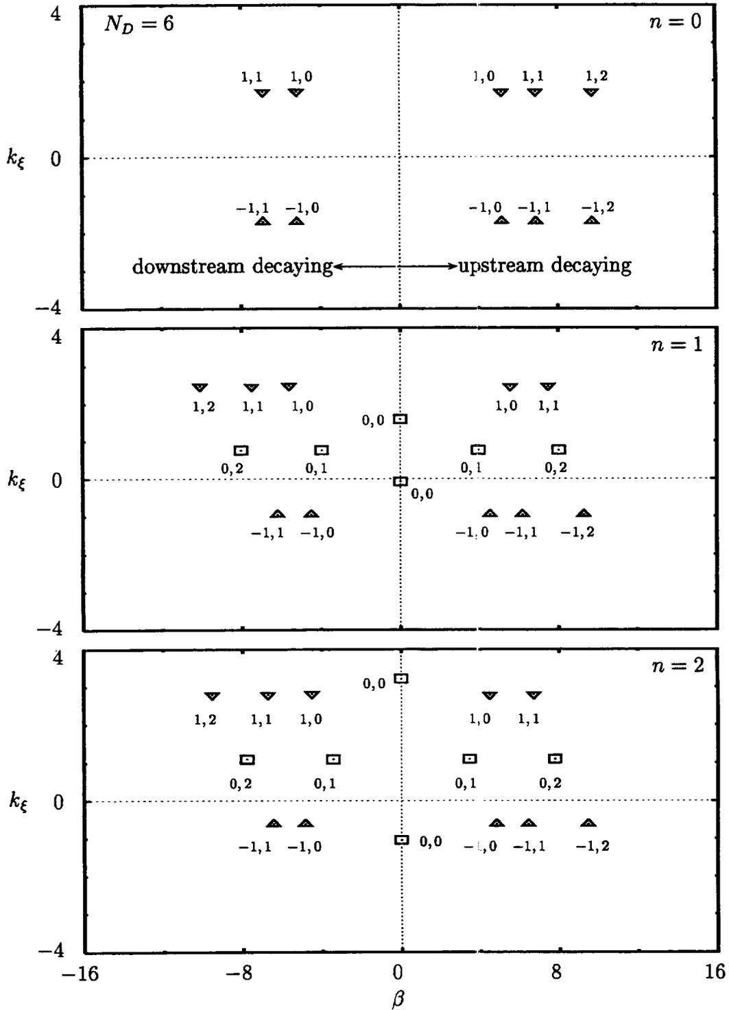
Figure 11: Axial eigenvalues,  $\chi = \beta + i\kappa_\xi$ , at inlet for three circumferential ( $m = -1, 0, 1$ ) and three radial ( $\mu = 0, 1, 2$ ) modes of steady ( $n = 0$ ), first-harmonic ( $n = 1$ ) and second-harmonic ( $n = 2$ ) acoustic disturbance in an unsteady flow at  $\omega = 1.0$  and  $N_D = 6$ , through the 3D 10th Standard Cascade.
