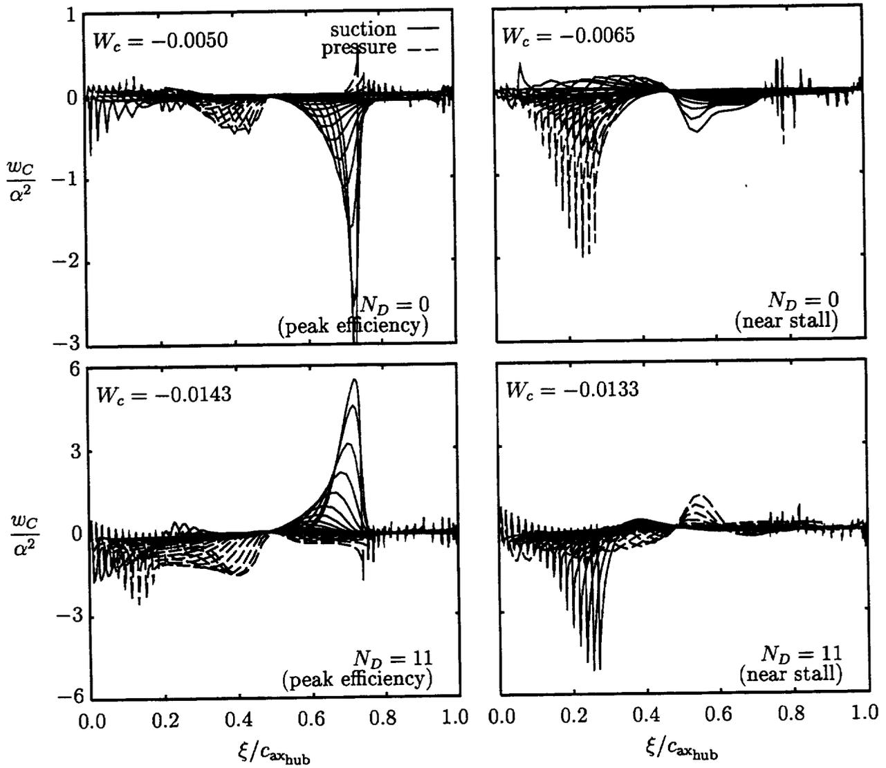
Figure 27: Local work per cycle distributions and global works per cycle for the Rotor 67 fan undergoing pure torsional vibrations about midchord at  $\omega = 0.54$  and  $\sigma = 0$  and  $180$  deg ( $N_D = 0$  and  $11$ ).
