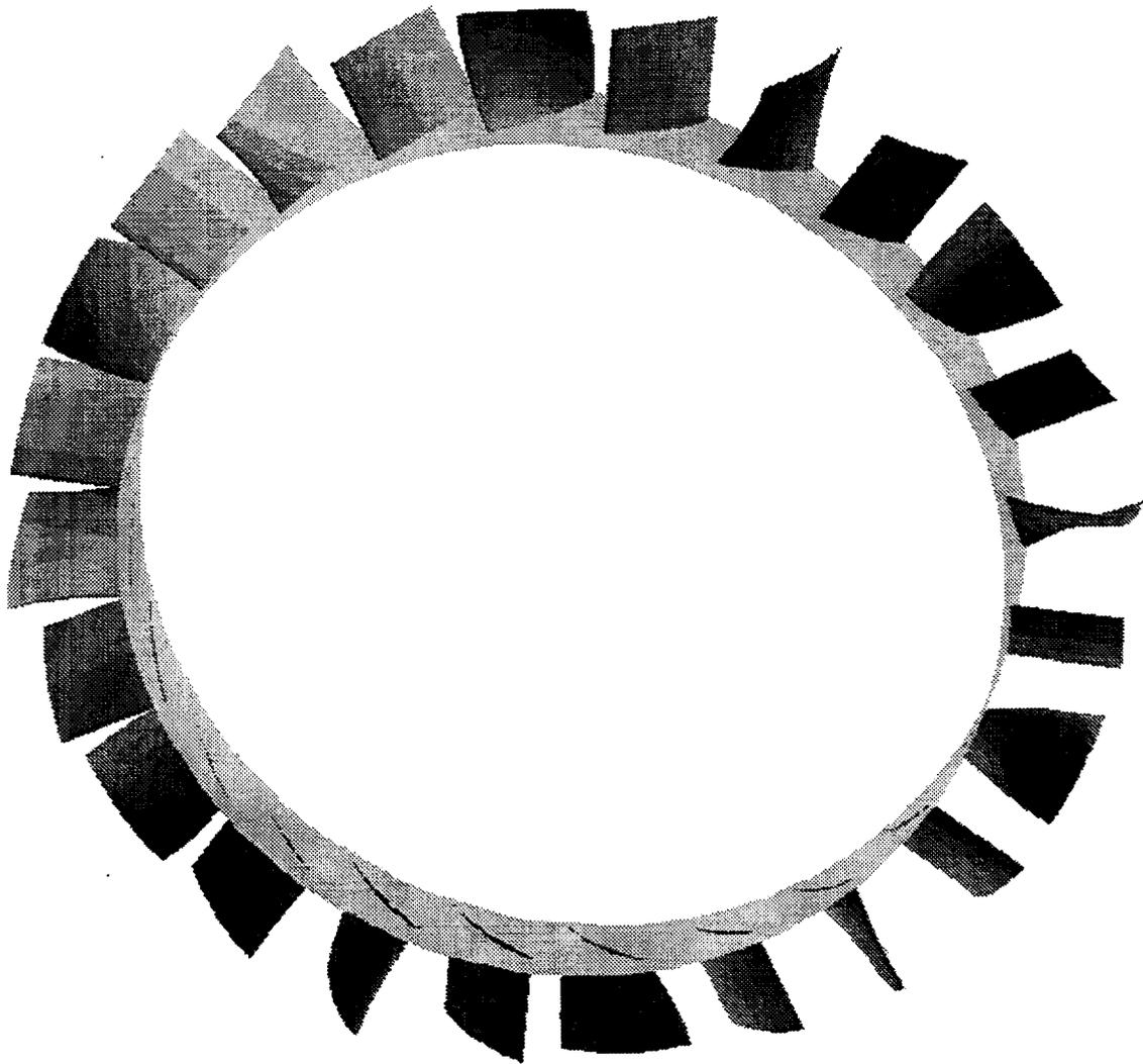
Figure 2: 3D Tenth Standard Configuration undergoing an exaggerated torsional motion ( $\alpha_{hub} = 0$  deg,  $\alpha_{tip} = 45$  deg). The rotor consists of 24 airfoils. The nodal diameter of the blade motion is 6, which results in an interblade phase angle of 90 deg. The outer casing has been eliminated from the figure for clarity.
