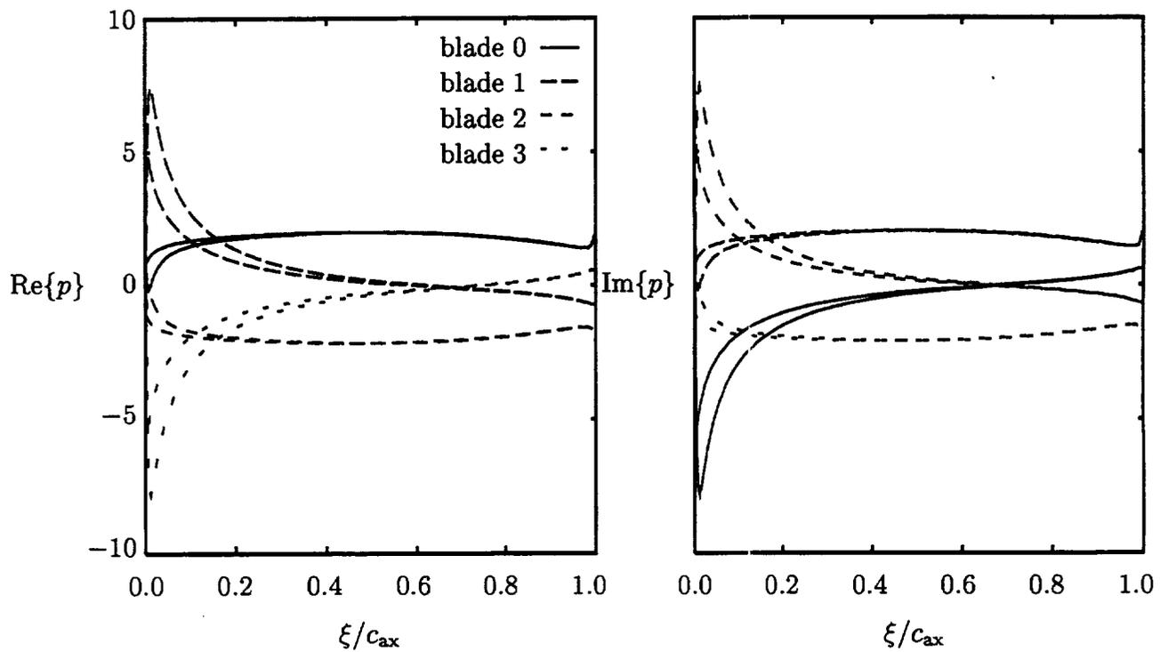
Figure 15: First-harmonic unsteady pressure distributions at midspan acting on four blades of the 3D 10th Standard Cascade undergoing a pure bending vibration at  $\omega = 1.0$  and  $N_D = -6$ .
