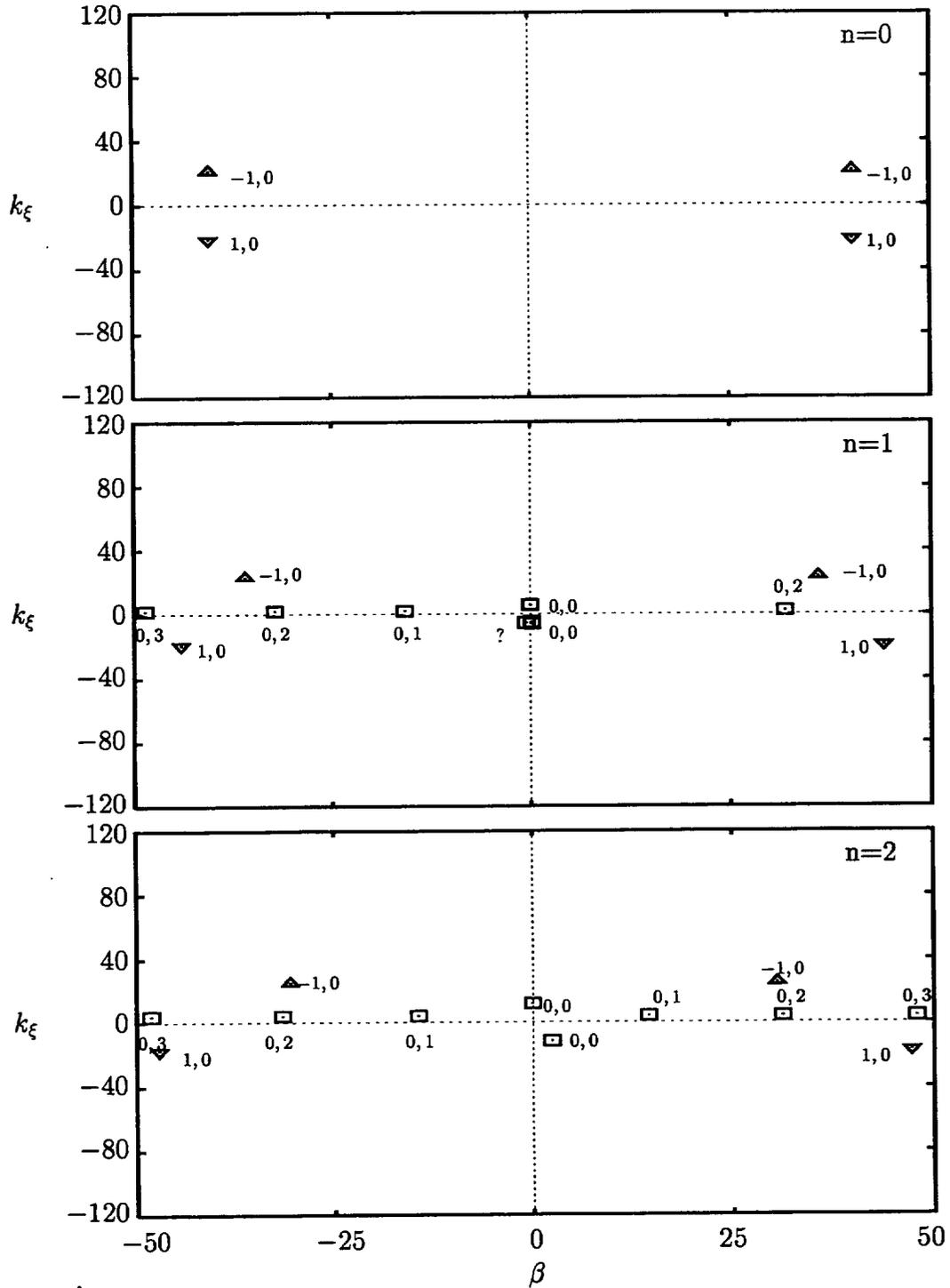
Figure 25: Axial eigenvalues,  $\chi = \beta + i\kappa_\xi$ , at exit for the time-mean ( $n = 0$ ), and the first ( $n = 1$ ) and second ( $n = 2$ ) temporal harmonics, and three circumferential ( $m = -1, 0, 1$ ) and five radial ( $\mu = 0, 1, 2, 3, 4$ ) modes of acoustic disturbance in the far field of Rotor 67, for an unsteady flow at  $\omega = 0.54$  and  $N_D = 0$ , and a meanflow condition near peak efficiency.
