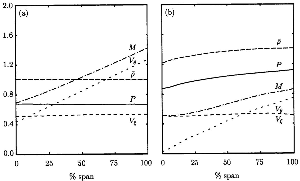
Figure 23: Relative frame steady flow properties (a) far upstream and (b) far downstream of the NASA Rotor 67 fan ( $M_{-\infty}^{abs} \approx 0.526$ ,  $|\Omega| = 2.524$ ).
