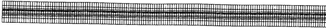
Figure 4. 2D cylinder long-wake computation at Re = 140 . Arrangement of the two subdomains. Frames do not show the actual mesh.
